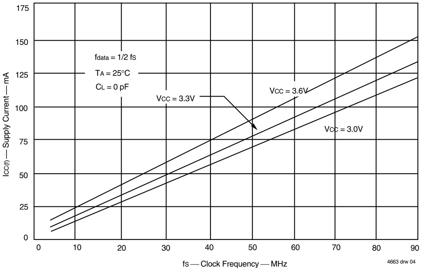
Figure 1. Typical Characteristics: Supply Current (I<sub>CC</sub>) vs. Clock Frequency (f<sub>s</sub>)
