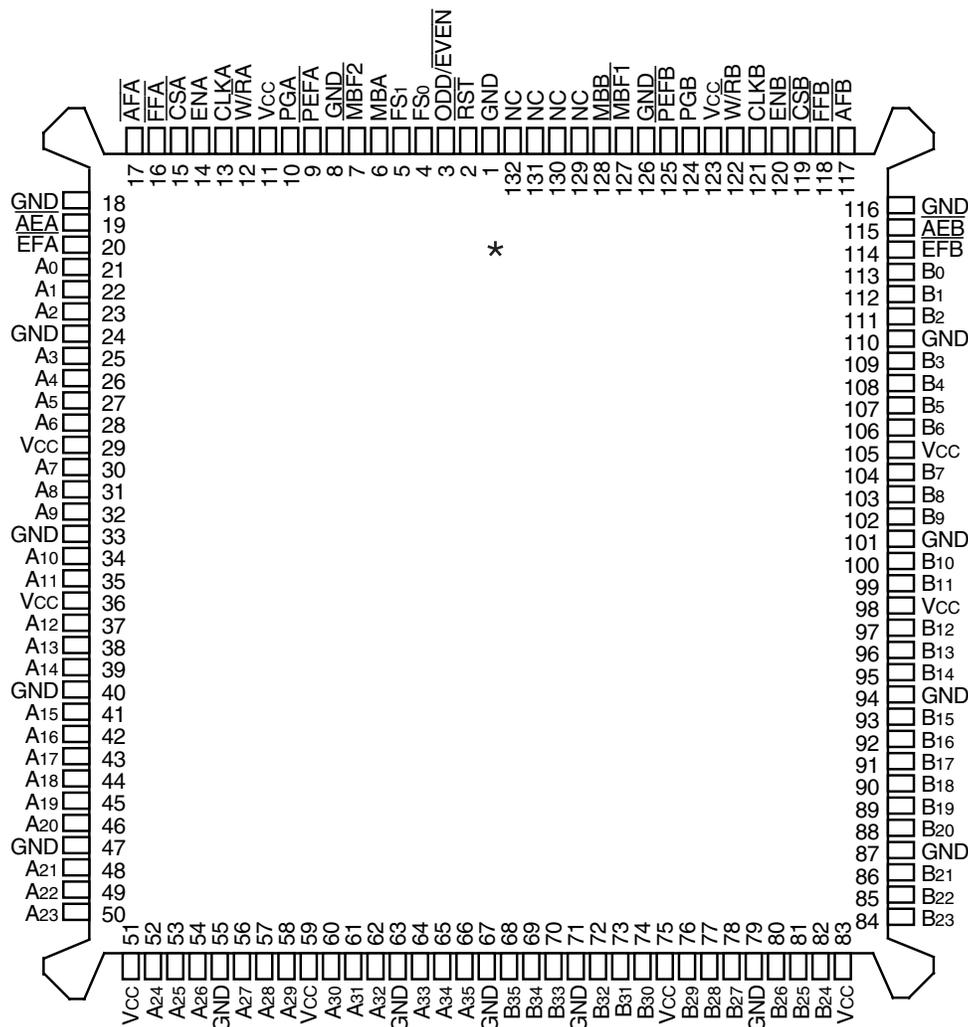
\* Electrical pin 1 in center of beveled edge. Pin 1 identifier in corner.
