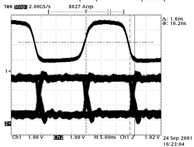
From the above measurements taken, the amount of jitter being added at each TX point is not significant. These tests were also run for extended periods of time (64 hours) and no bit errors were seen.
