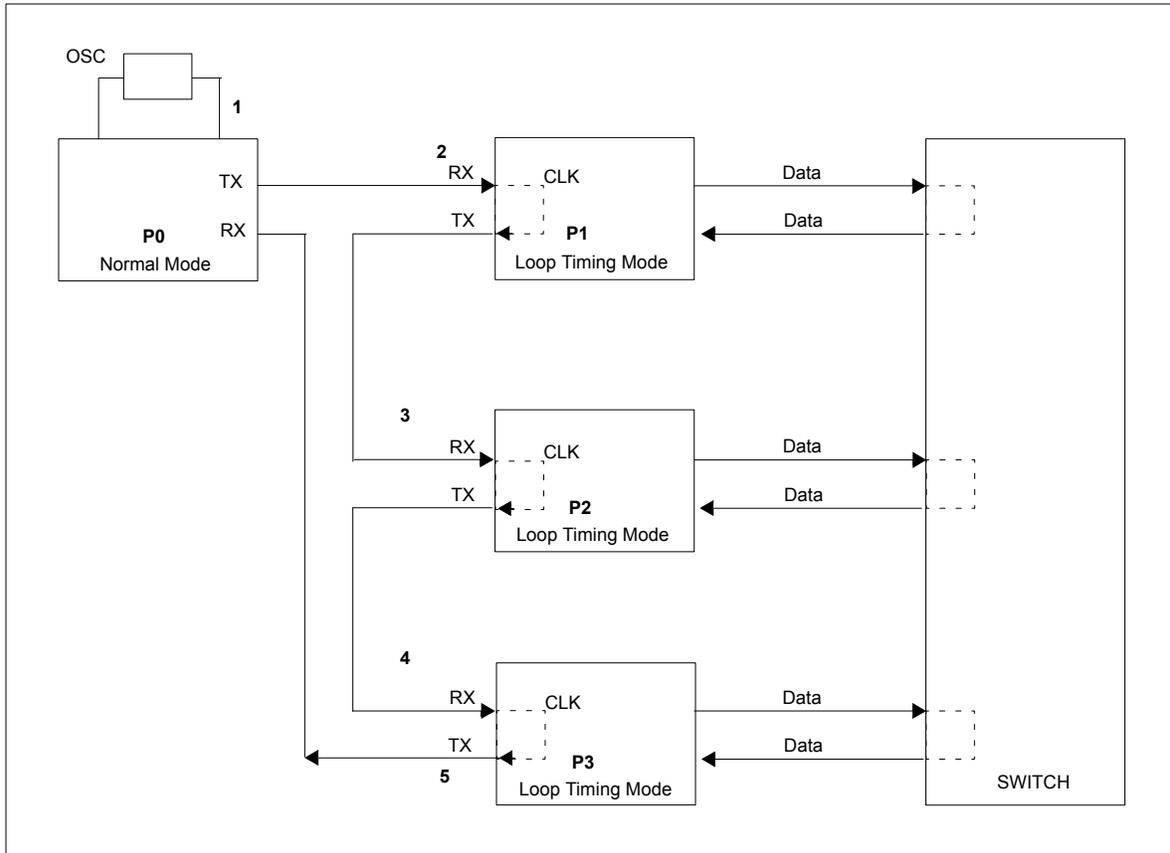
Figure 35 Test Setup for Loop Timing Jitter Measurements
