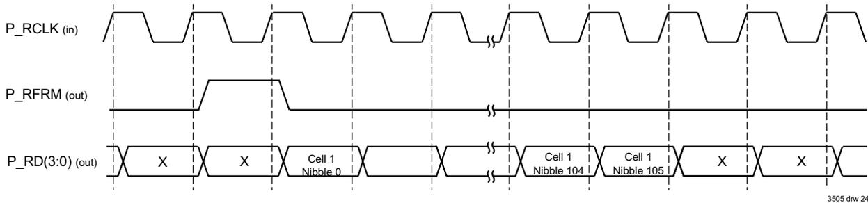
Figure 23 DPI Receive Handshake - One Cell Received
