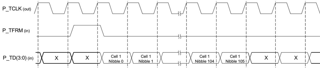
Figure 27 DPI Transmit Handshake - One Cell for Transmission
