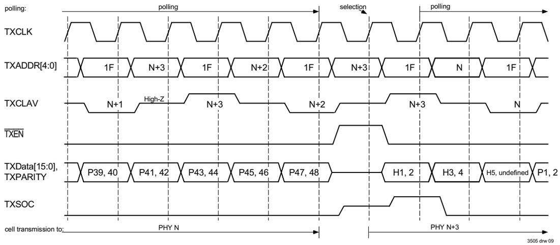
Figure 9 Utopia 2 Transmit Handshake - Back to Back Cells
