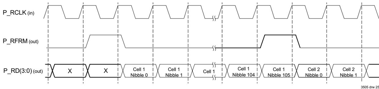
Figure 24 DPI Receive Handshake - Back-to-Back Cells
