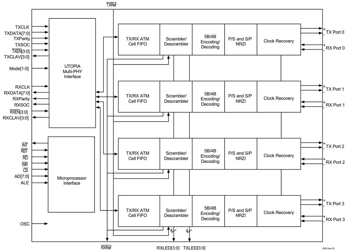
Figure 2 Block Diagram for Utopia Level 1 Configuration (MODE[1:0] = 01)
