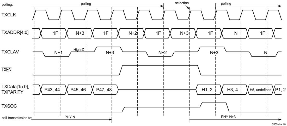
Figure 10 Utopia 2 Transmit Handshake - Delay Between Cells
