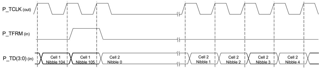
Figure 29 DPI Transmit Handshake - 77V1254L25 Transmit FIFO Full
