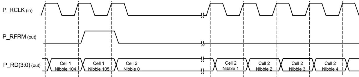
Figure 25 DPI Receive Handshake - ATM Layer Device Suspends Transfer
