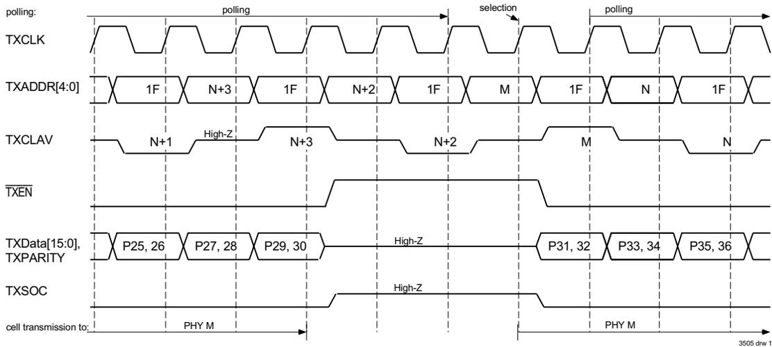
Figure 11 Utopia 2 Transmit Handshake - Transmission Suspended
