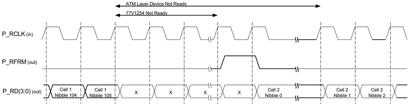
Figure 26 DPI Receive Handshake - Neither Device Ready
