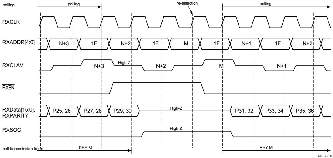
Figure 14 Utopia 2 Receive Handshake - Suspended Transfer of Data
