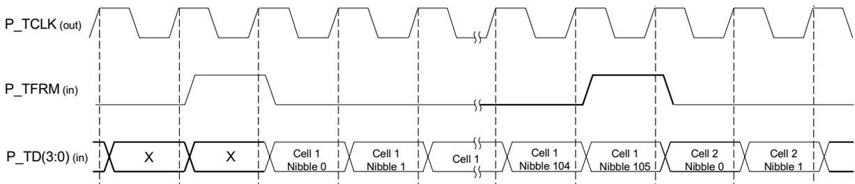
Figure 28 DPI Transmit Handshake - Back-to-Back Cells for Transmission
