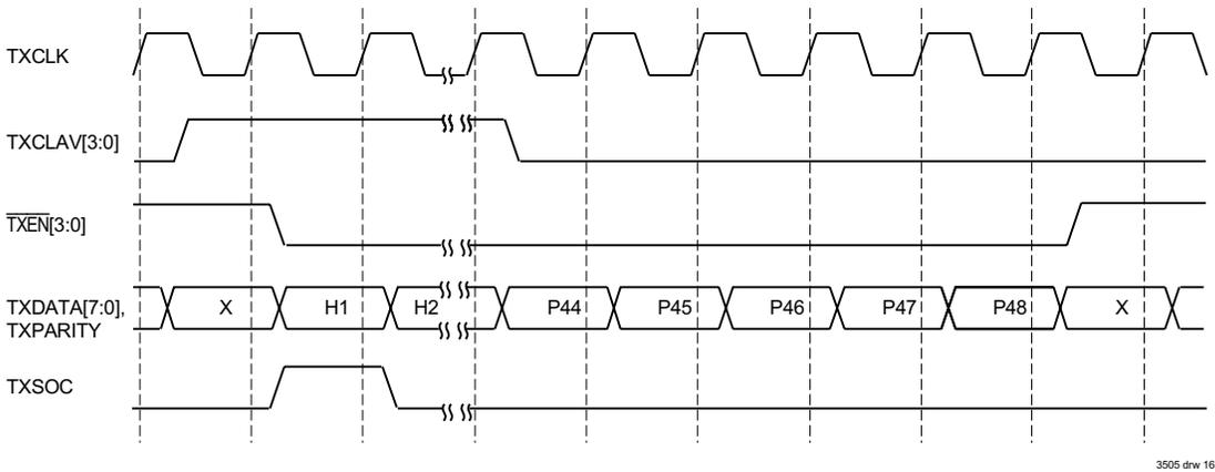
Figure 15 Utopia 1 Transmit Handshake - Single Cell
