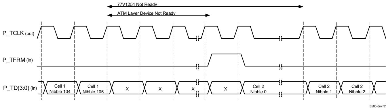
Figure 30 DPI Transmit Handshake - Neither Device Ready
