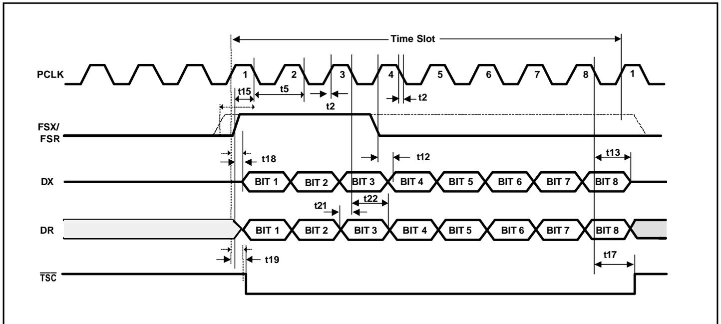
Figure 4. PCM Interface Timing for Long Frame Mode
