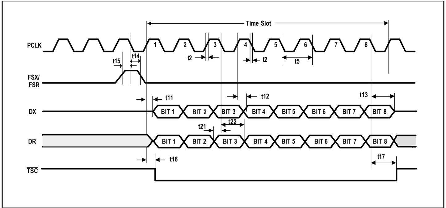
Figure 3. PCM Interface Timing for Short Frame Mode
