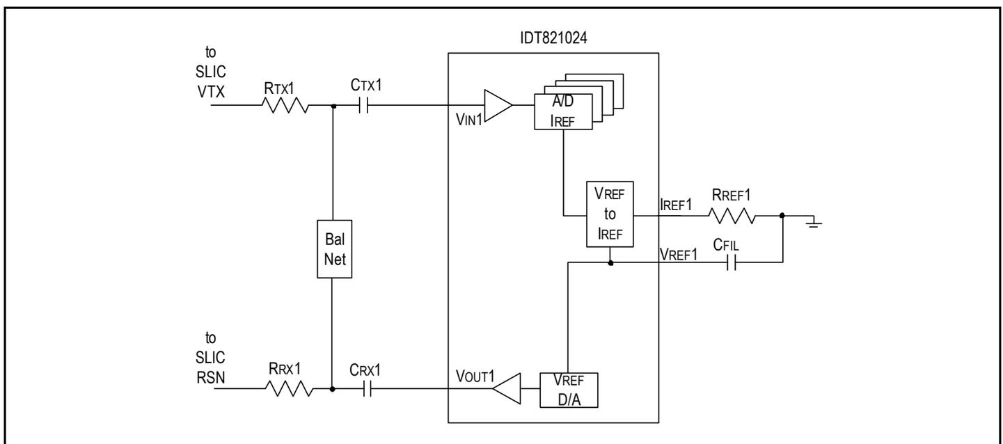
Figure 1. IDT821024 Transmit Gain Setting for Channel 1
