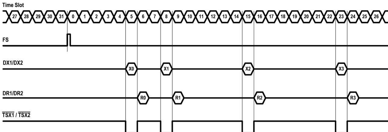
Figure - 12 Typical Frame Sync Timing (2 MHz Operation)
