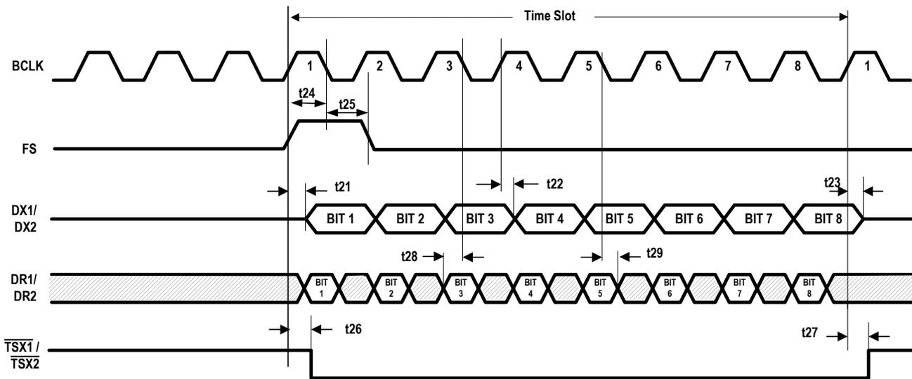
Note: This timing diagram only applies to the situation of receiving data on falling edges and transmitting data on rising edges.
