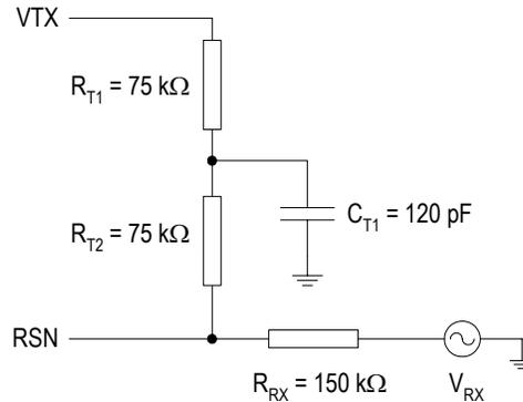
Figure 6 Two-Wire AC Input Impedance Programming Network
