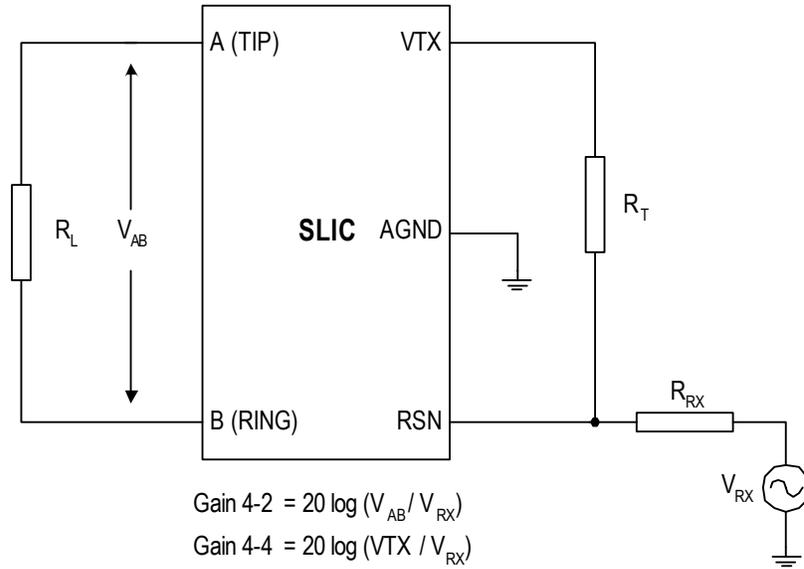
Figure 11 Four-to-Two Wire Gain and Four-to-Four Wire Gain
