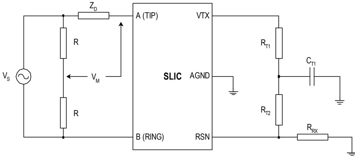
$Z_D$ : The desired impedance (e.g., the characteristic impedance of the line)
