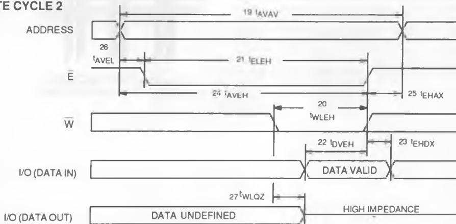
WRITE CYCLE 2 waveform shows a write cycle terminated by  $\bar{E}$  going high. Data set-up and hold times are referenced to the rising edge of  $\bar{E}$ . With  $\bar{E}$  high, the outputs remain in the high impedance state.
