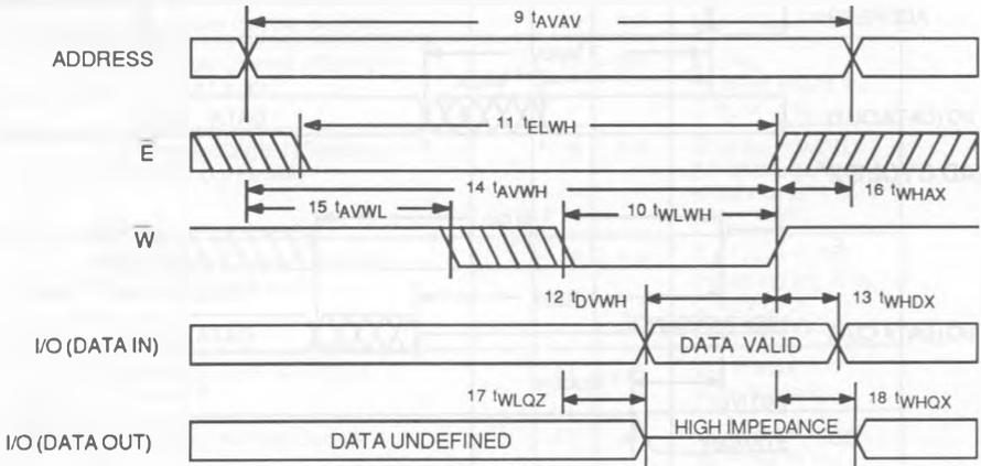
The READ CYCLE 2 waveform shows a read access that is initiated by  $\bar{E}$  going low. As long as address is stable when  $\bar{E}$  goes low, valid data is at the output at the specified Chip Enable Access time. If address is not valid when  $\bar{E}$  goes low, the timing is as specified in READ CYCLE 1. Chip Enable access time is not affected by the duration of the deselect interval.
