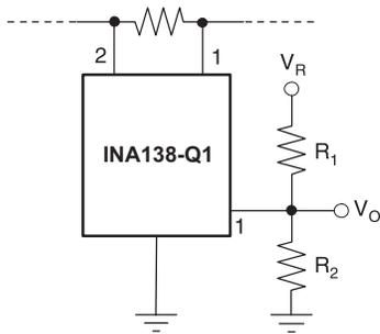
Gain Set by  $R_1 \parallel R_2$
