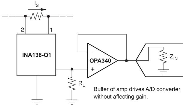
**Figure 10. Buffering Output to Drive and A/D Converter**
