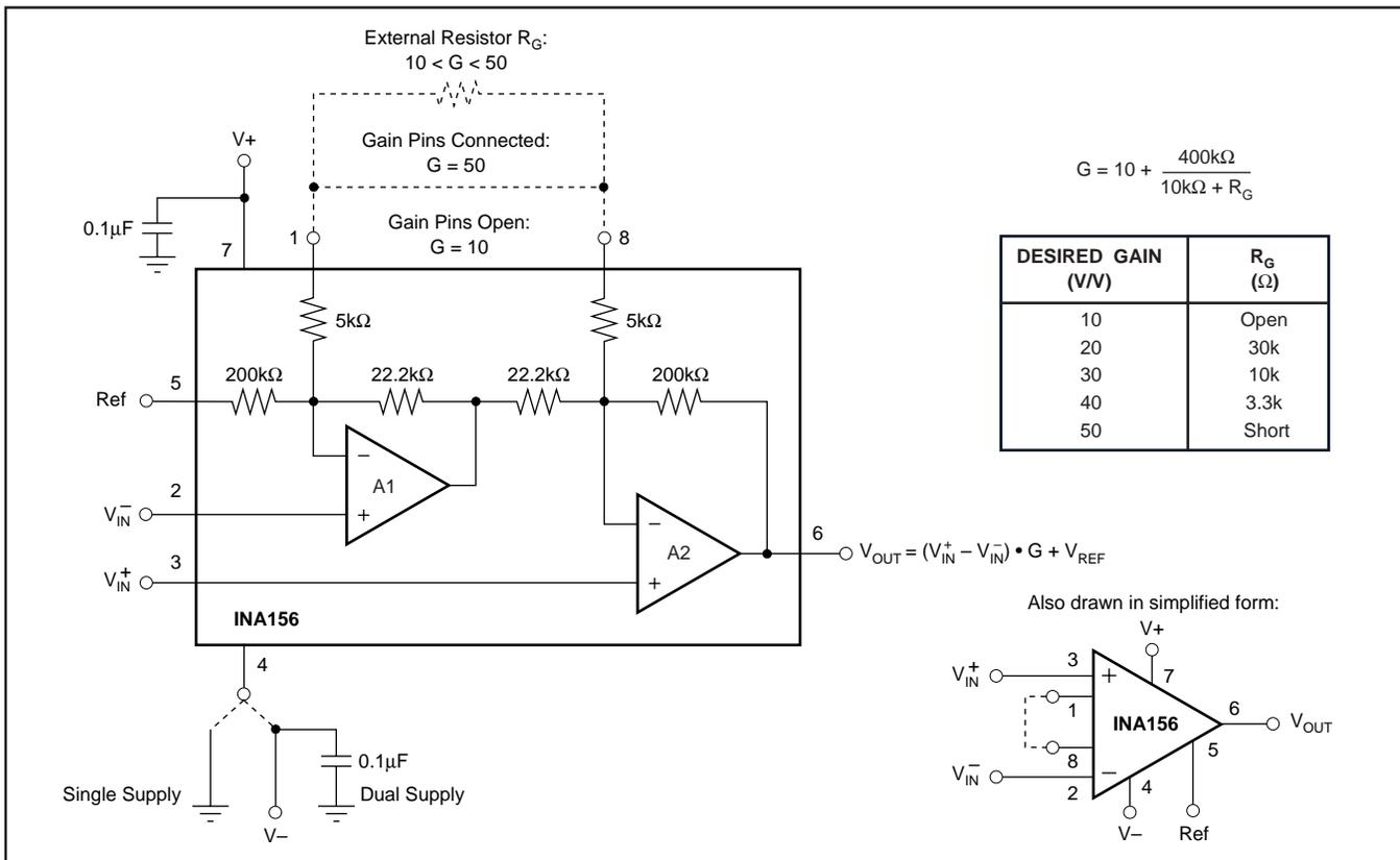
FIGURE 1. Basic Connections.
