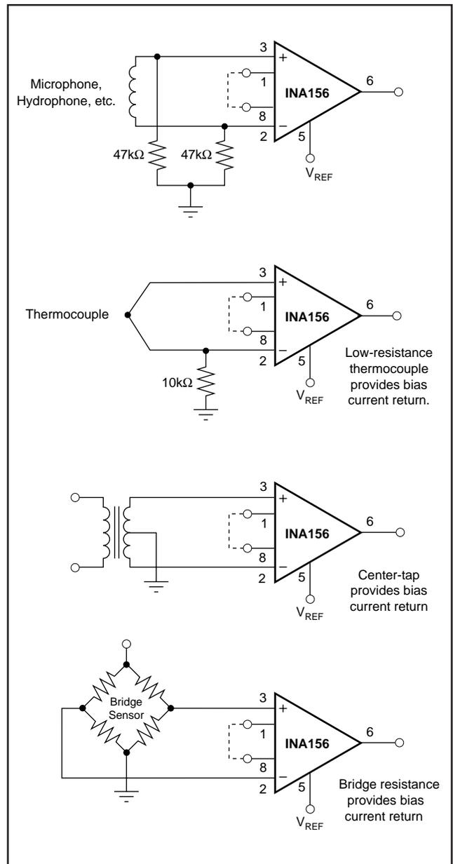
FIGURE 5. Providing an Input Common-Mode Current Path.
