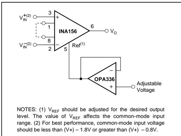
FIGURE 4. Optional Trimming of Output Offset Voltage.
