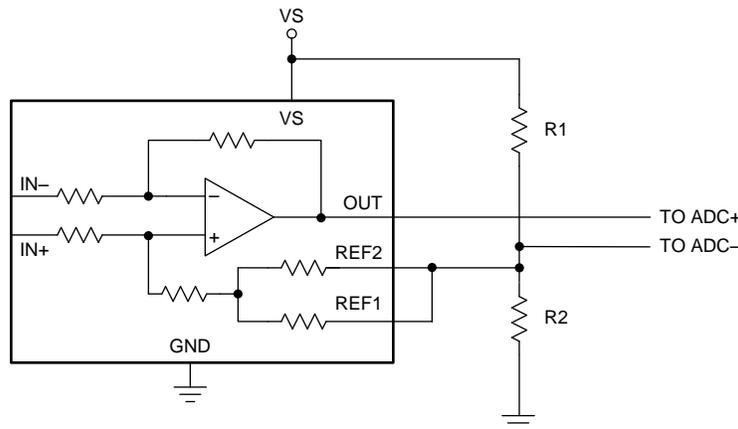
Figure 31. Setting the Reference Using a Resistor Divider
