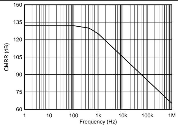
Figure 12. Common-Mode Rejection Ratio vs Frequency
