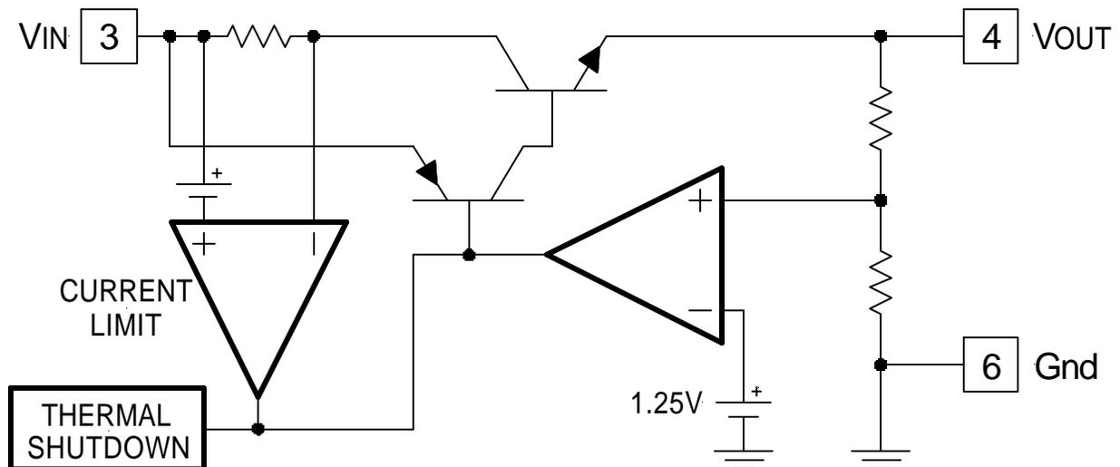
Figure 2 - Simplified block diagram of the IRU1011-33.
