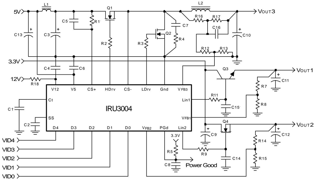
Figure 3 - Typical application of IRU3004 in an on-board DC-DC converter providing the Core, GTL+, and Clock supplies for the Pentium II microprocessor.
