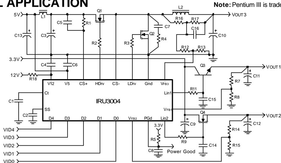
Figure 1 - Typical application of the IRU3004.
