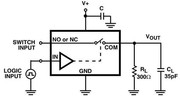
$C_L$  includes fixture and stray capacitance.
