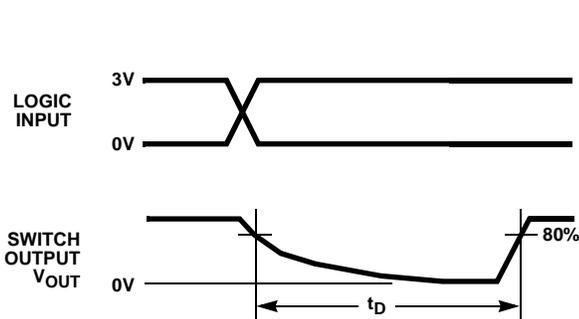
FIGURE 3A. MEASUREMENT POINTS
