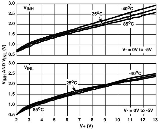
FIGURE 17. DIGITAL SWITCHING POINT vs POSITIVE SUPPLY VOLTAGE
