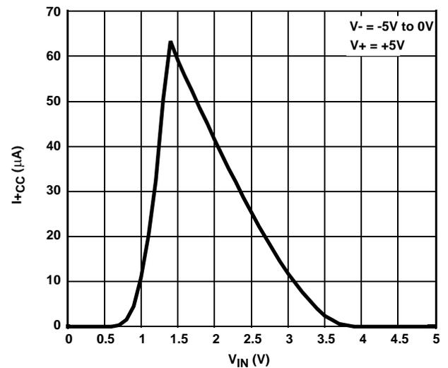
FIGURE 18. POSITIVE SUPPLY CURRENT vs DIGITAL INPUT VOLTAGE
