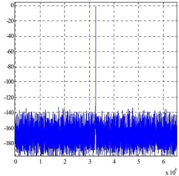
FIGURE 20. A TYPICAL SPECTRUM PLOT (65536 POINT FFT, BLACKMAN WINDOW, 800 Hz BIN NBW (29 dB). PEAK BIN IS AT -132 dBc, NOISE FLOOR AT -190 dBc/Hz.)
