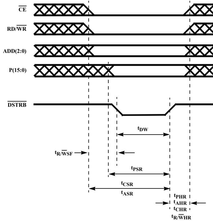
FIGURE 15. MICROPROCESSOR WRITE TIMING ( $\mu\text{P}$  mode = 1))
