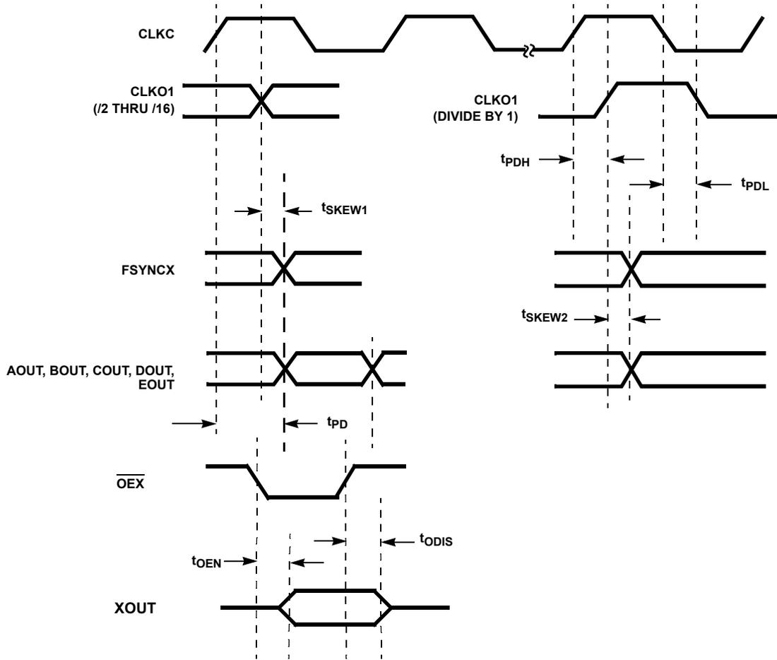
FIGURE 18. OUTPUT TIMING
