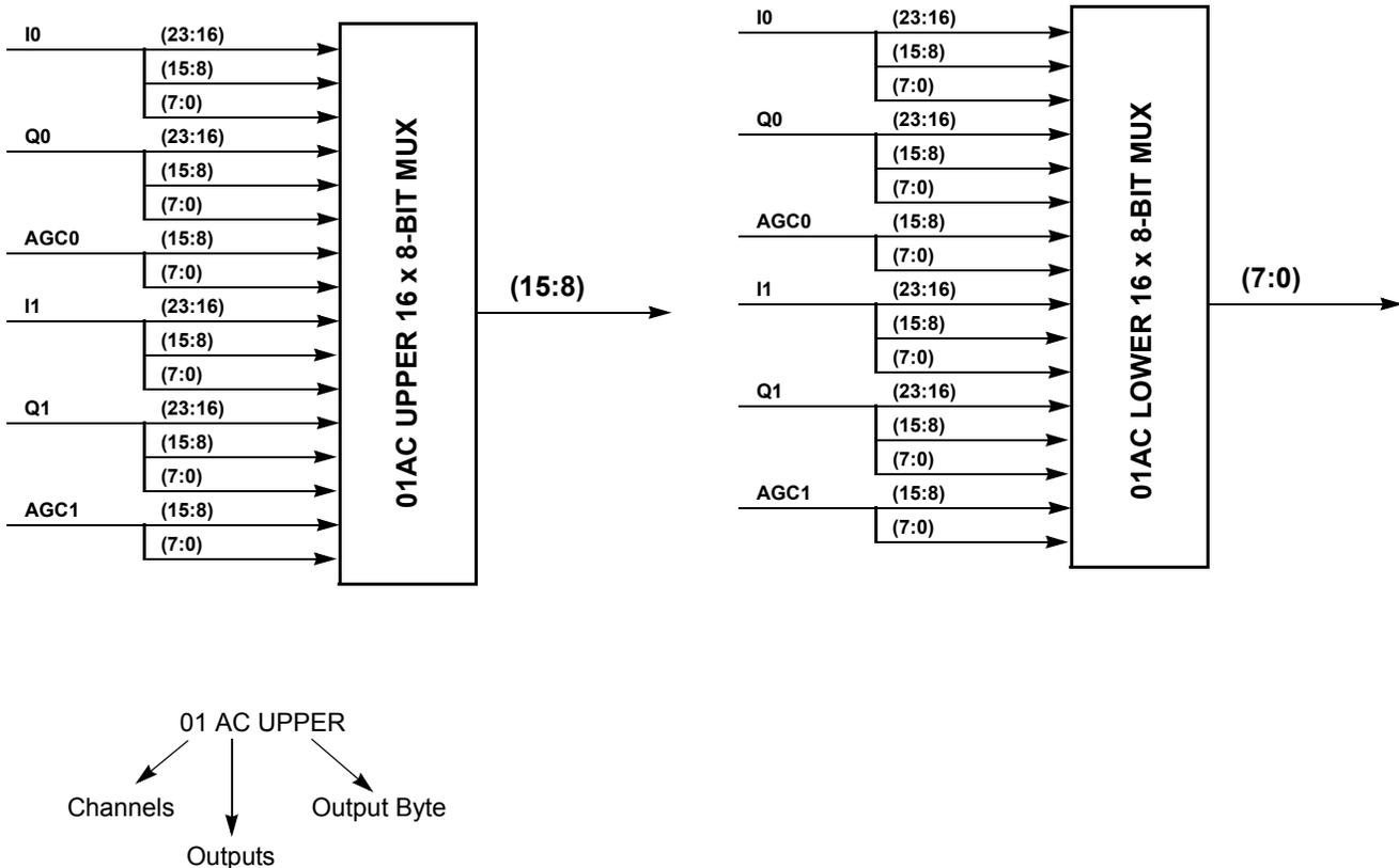
FIGURE 9. MULTIPLEXING CHANNELS
