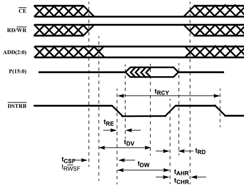
FIGURE 16. MICROPROCESSOR READ TIMING ( $\mu\text{P}$  mode = 1))
