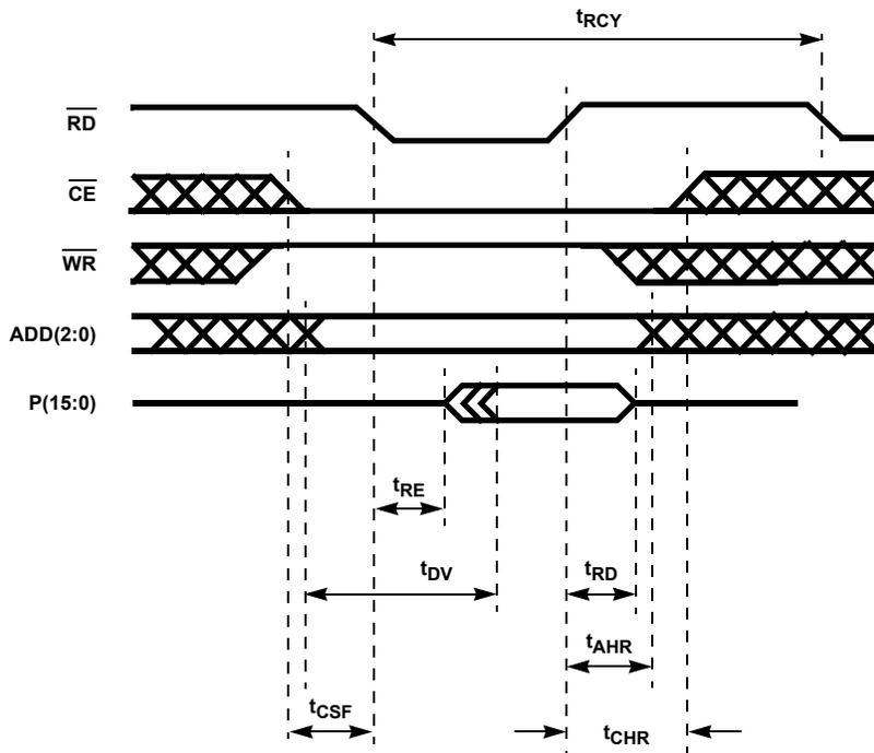
FIGURE 14. MICROPROCESSOR READ TIMING ( $\mu P$  mode = 0)
