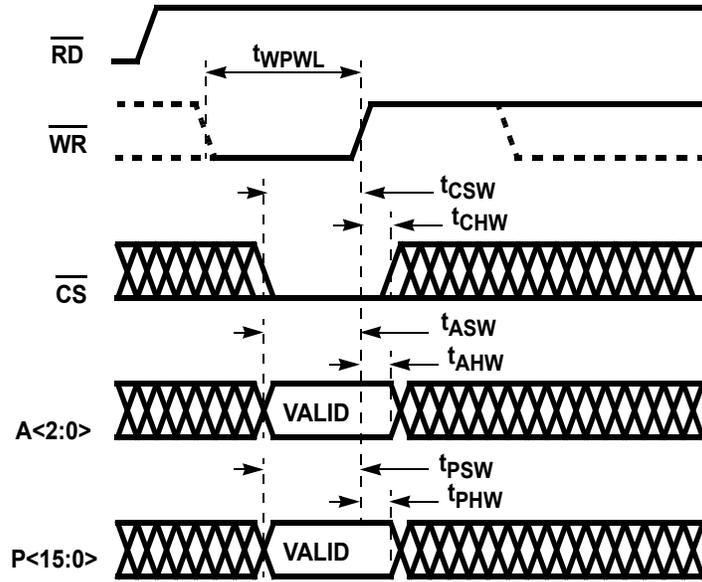
FIGURE 13. MICROPROCESSOR WRITE TIMING ( $\mu P$  mode = 0)
