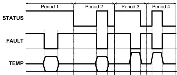
FIGURE 5. EFFECTS OF THE TEMP PIN.
