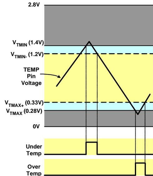
FIGURE 4. CRITICAL VOLTAGE LEVELS FOR TEMP PIN.
