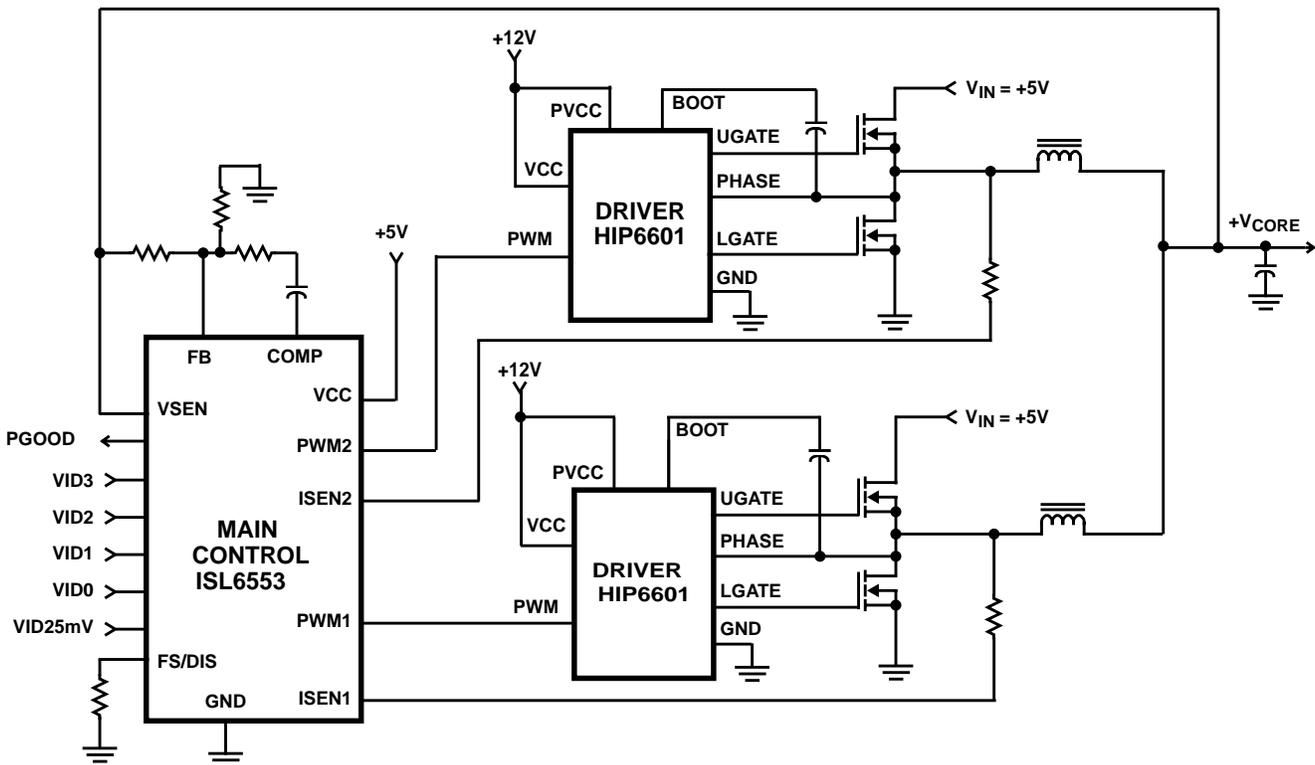
Typical Application - Two Phase Converter Using an HIP6602 Gate Driver
