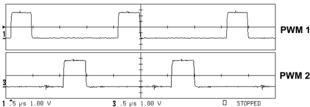
FIGURE 2. TWO PHASE PWM OUTPUT AT 500kHz
