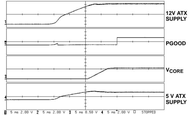
V<sub>IN</sub> = 5V, CORE LOAD CURRENT = 31A
