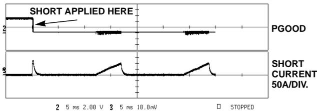
HICUP MODE. SUPPLY POWERED BY ATX SUPPLY
