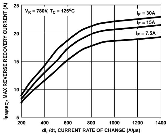
Figure 6. Maximum Reverse Recovery Current vs  $di_F/dt$
