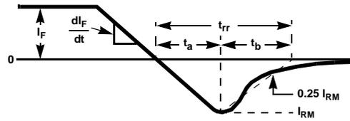
Figure 14.  $t_{tr}$  Waveforms and Definitions
