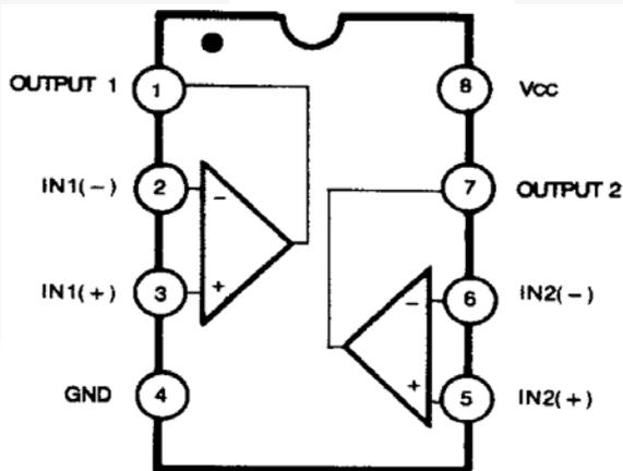
Figure 3. Block Diagram
