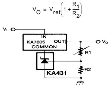
Figure 13. Output Control for Three-Terminal Fixed Regulator
