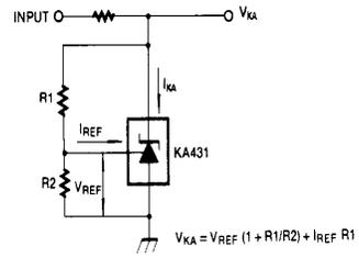
Figure 3. Test Circuit for  $V_{KA} \geq V_{REF}$
