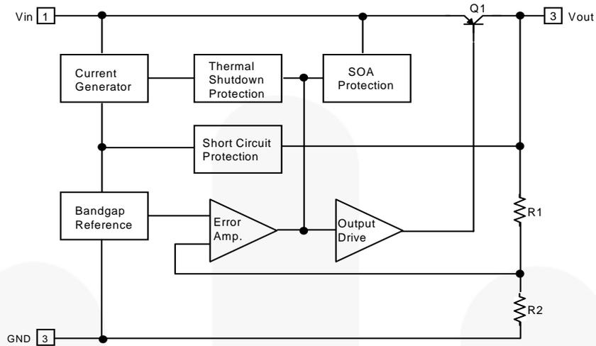
Figure 1. Block Diagram
