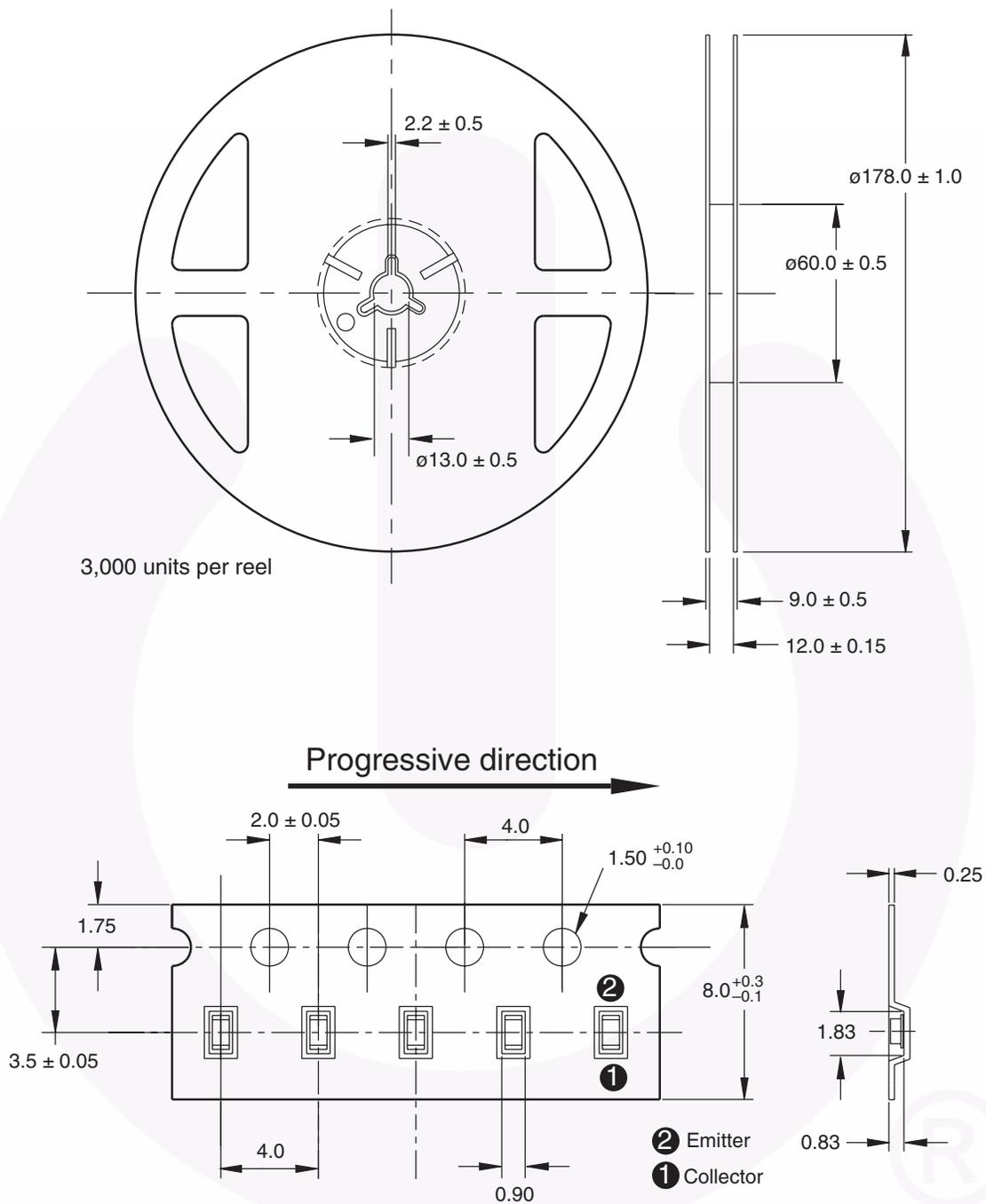
**Note:** Tolerances are  $\pm 0.1$ mm unless otherwise stated. All dimensions in mm.
