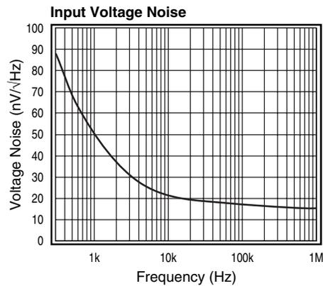
**KM4100/KM4101 Performance Characteristics** ( $V_s = +5V$ ,  $G = 2$ ,  $R_f = 2k\Omega$ ,  $R_L = 2k\Omega$  to  $V_s/2$ ; unless noted)
