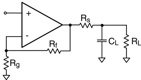
Figure 5: Typical Topology for driving a capacitive load
