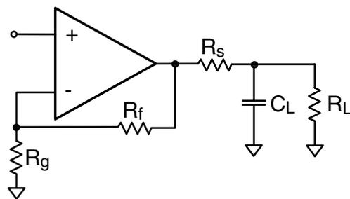
**Figure 4: Typical Topology for driving a capacitive load**
