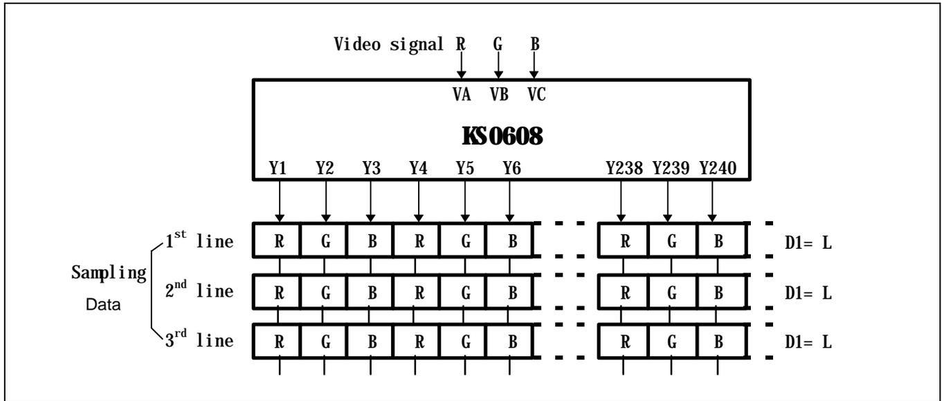
Video signal input pin connection.
