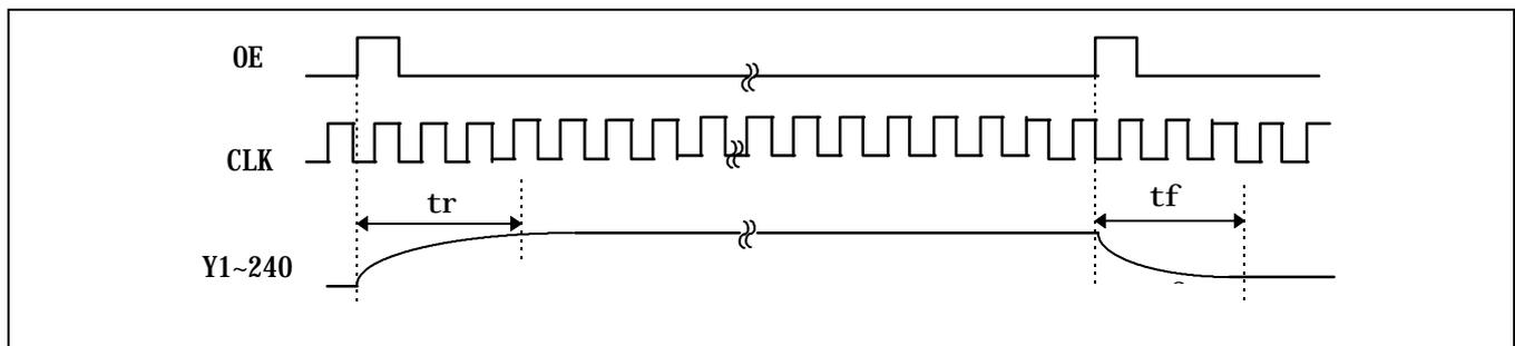
Start to output new data level at rising edge of OE Settling time  $t_r$ ,  $t_f$ , be controlled by VBS
