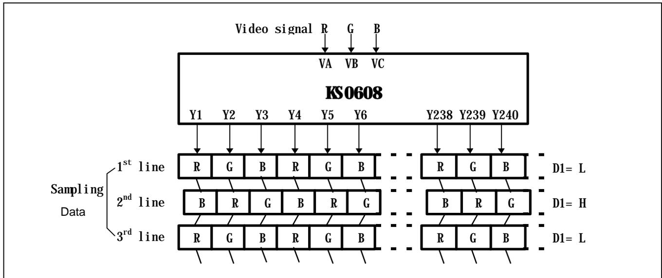
Video signal input pin connection.
