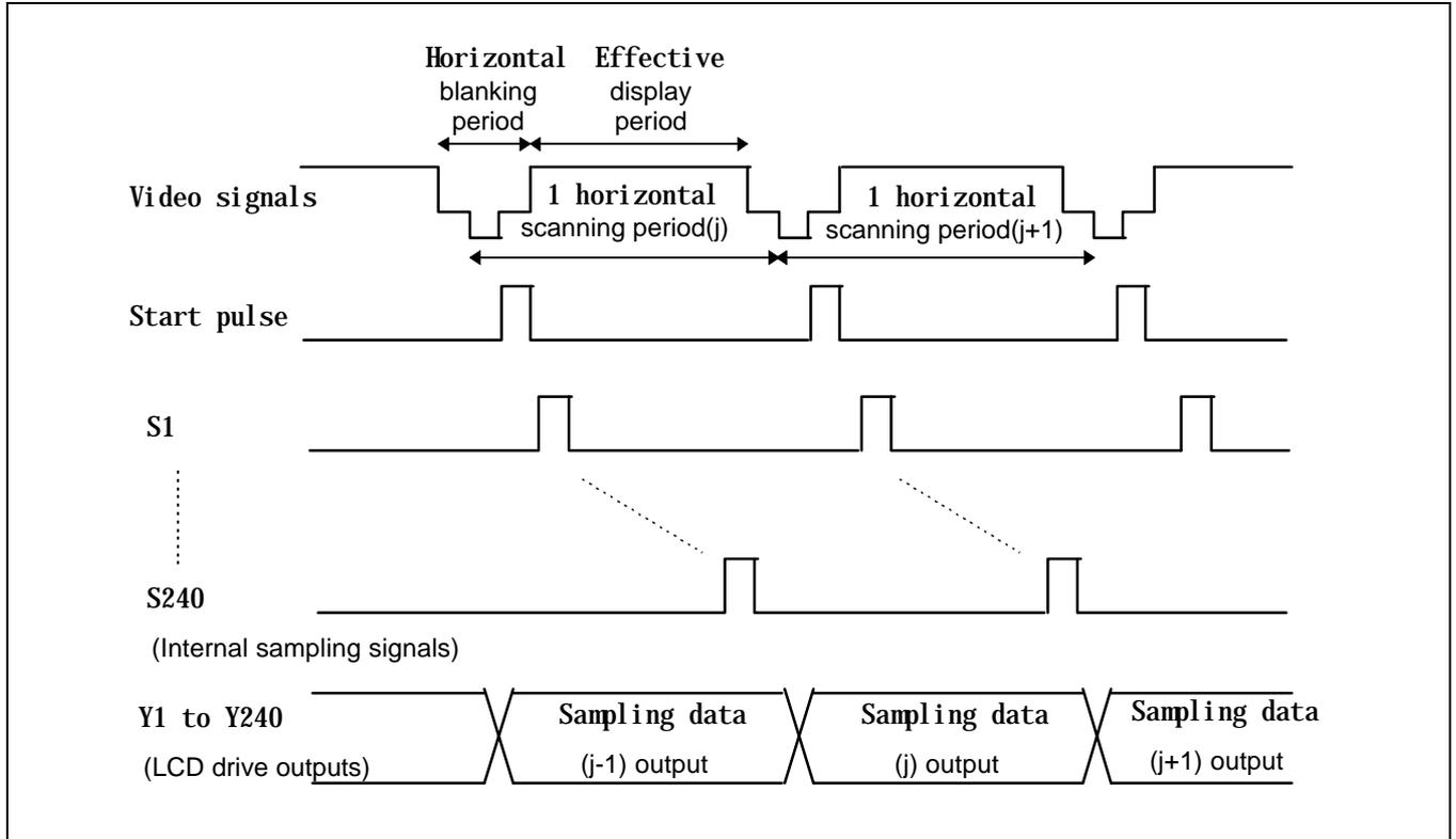
Samples a video signal based on the internal sampling pulse timing during 1 horizontal scanning period in each sample and hold circuit of the output circuit and outputs values corresponding to the sampling data.
