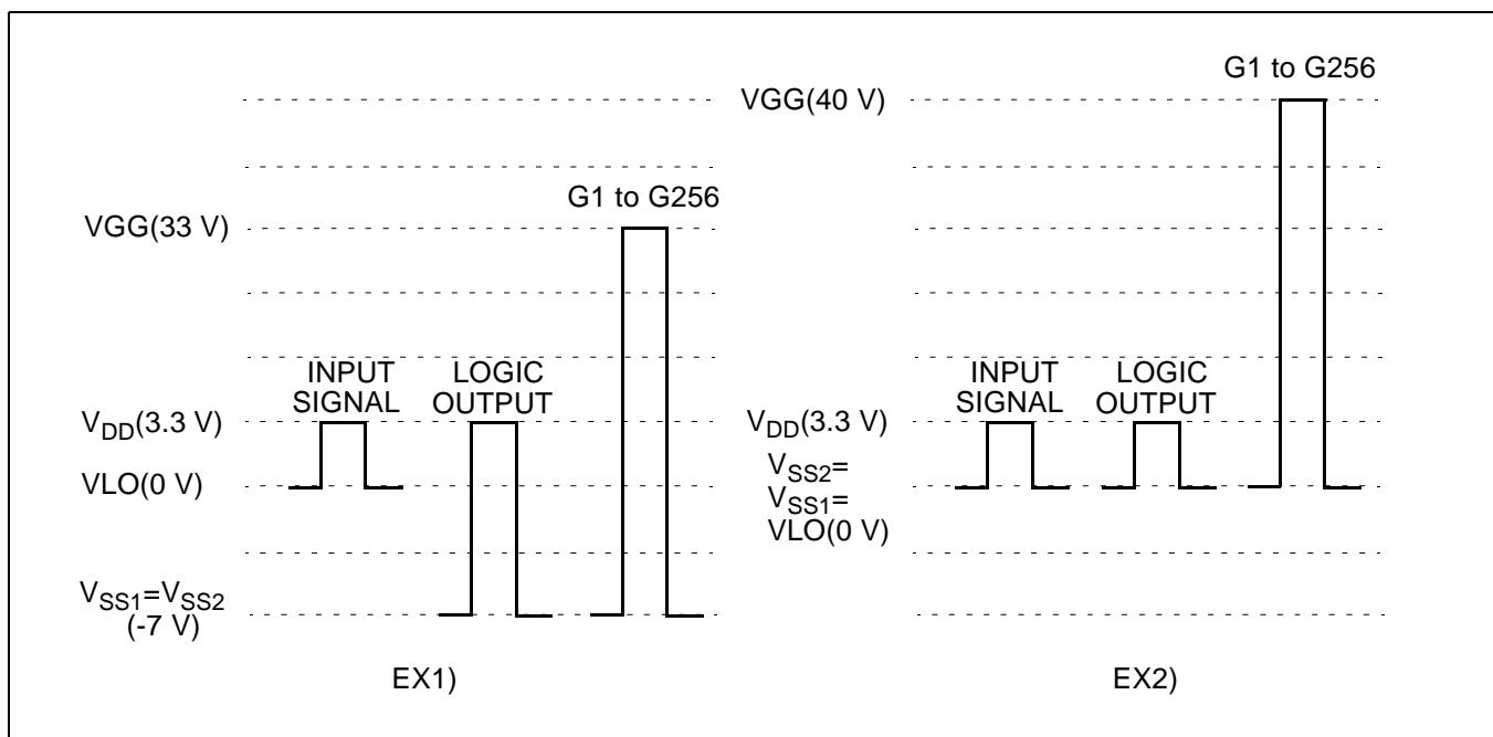
— Input signal (DI/O, DO/I, CPV, OE1 to 3) swings from VIL to VIH.
