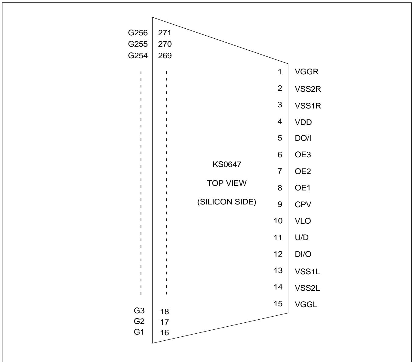
**NOTE:** Input pin arrangement in TCP can be modified (If the customer wants)
