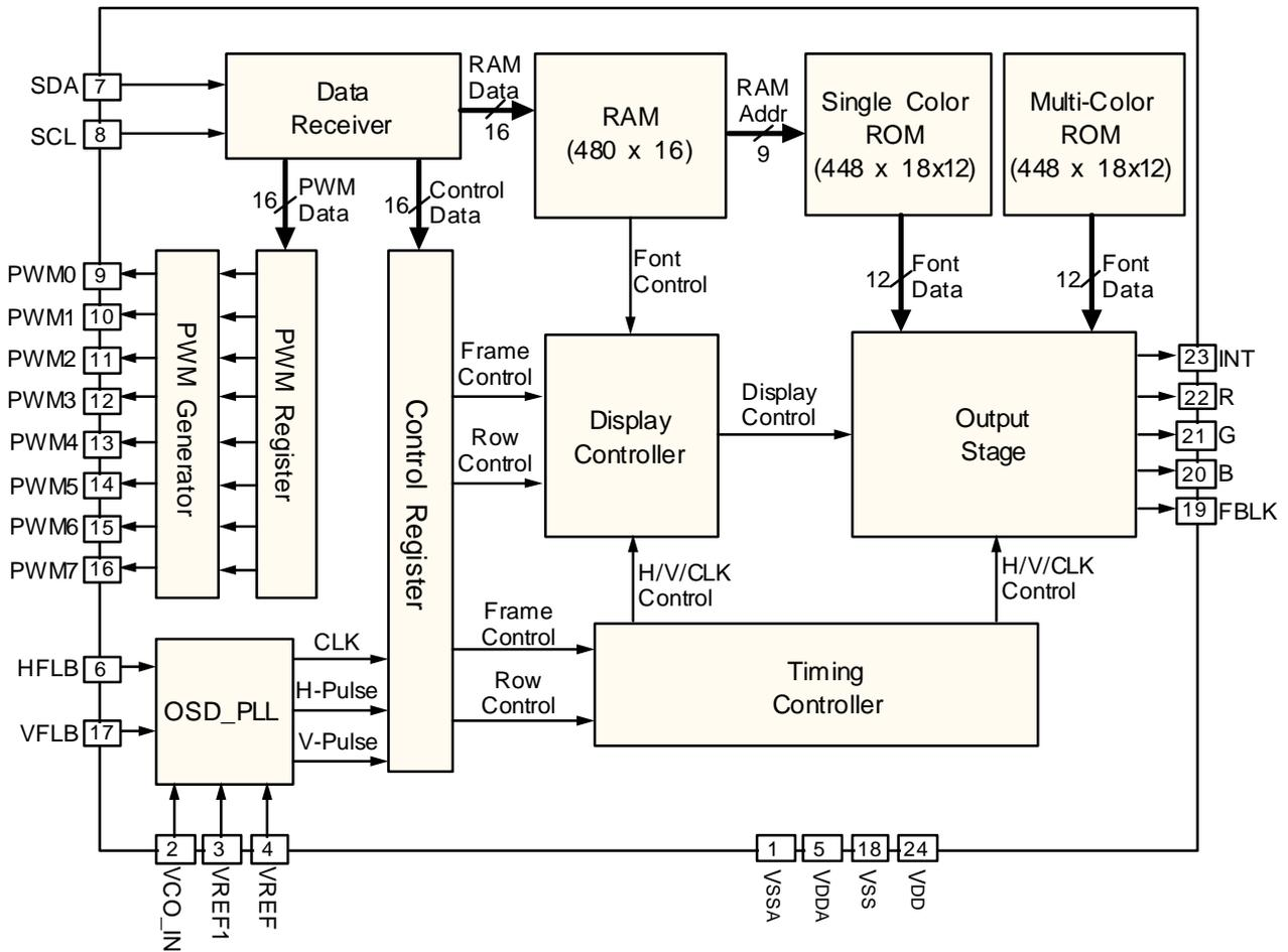
**Figure 1. Functional Block Diagram of KS2501**
