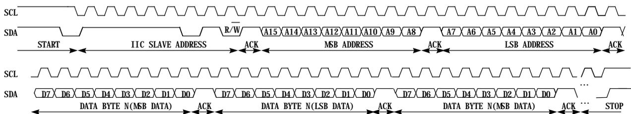
**Figure 4. SDA line and SCL line (Write Operation)**
