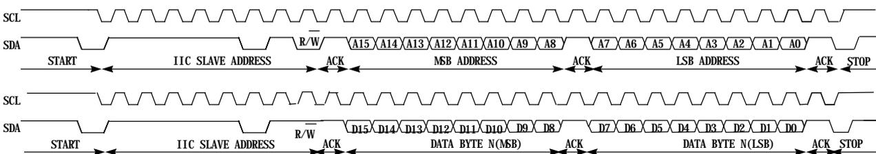
**Figure 5. SDA line and SCL line (Read Operation)**
