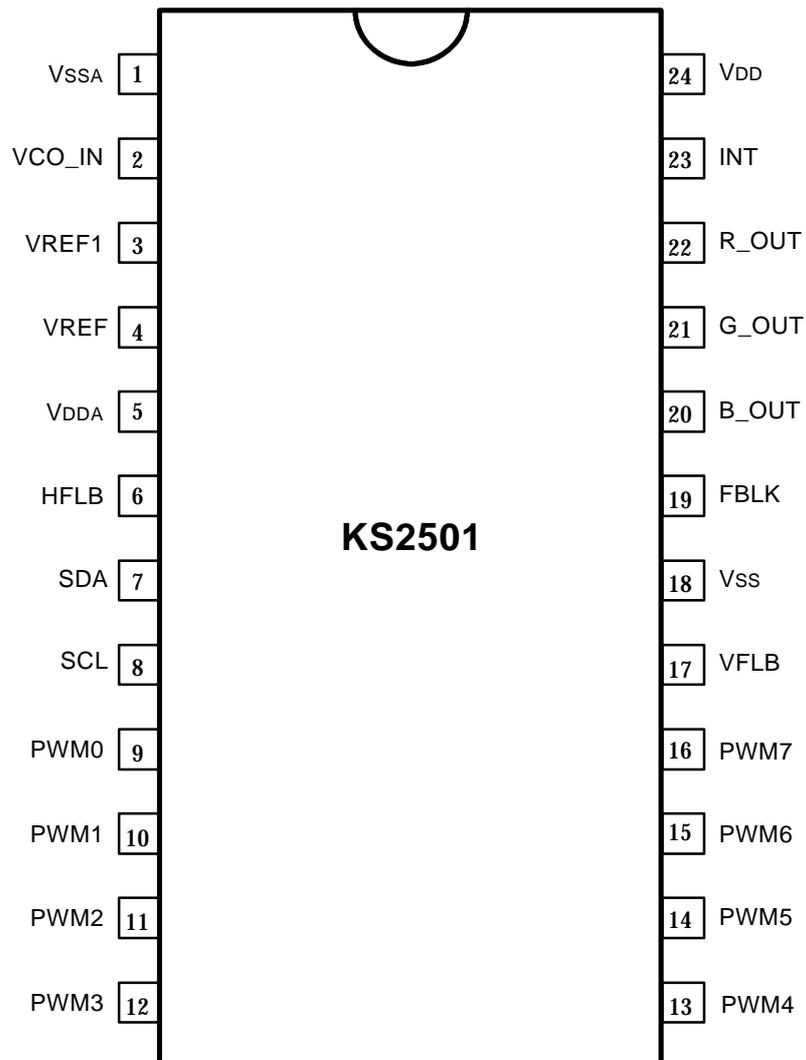
Figure 2. Pin Configurations
