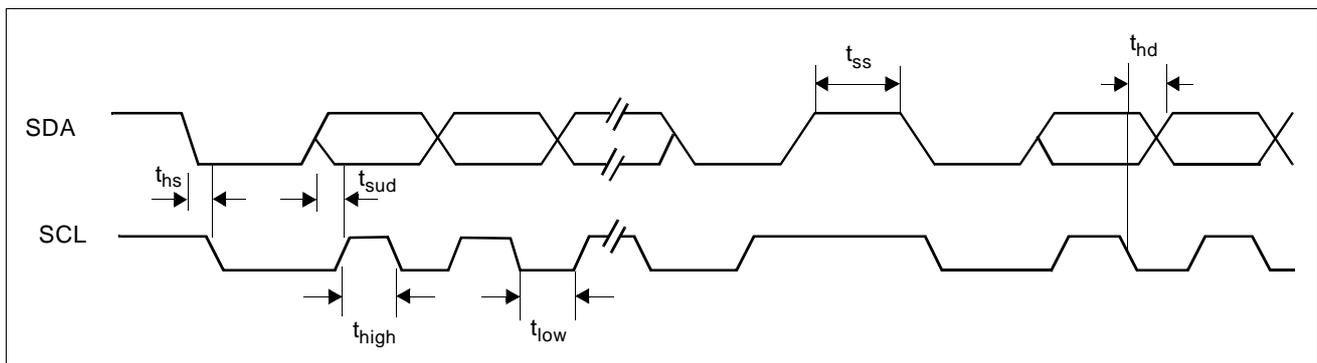
**Figure 3. I<sup>2</sup>C Bus Timing Diagram**
