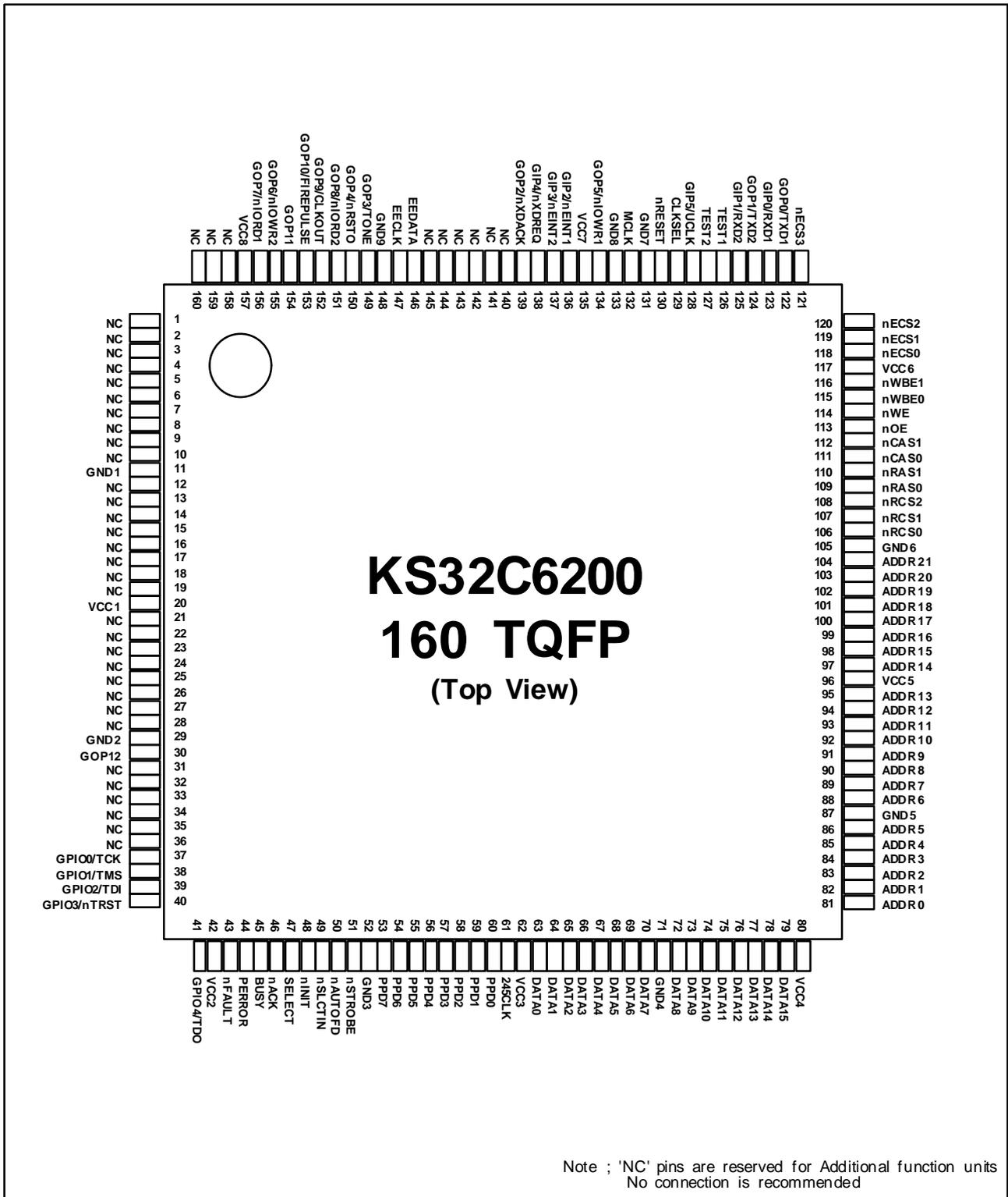
FIGURE 2. KS32C6200 PIN ASSIGNMENTS
