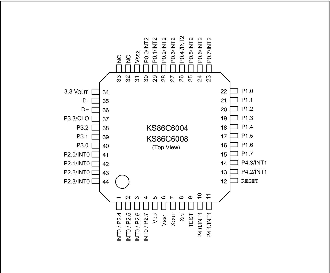
Figure 1-3. Pin Assignment Diagram (44-Pin QFP Package)
