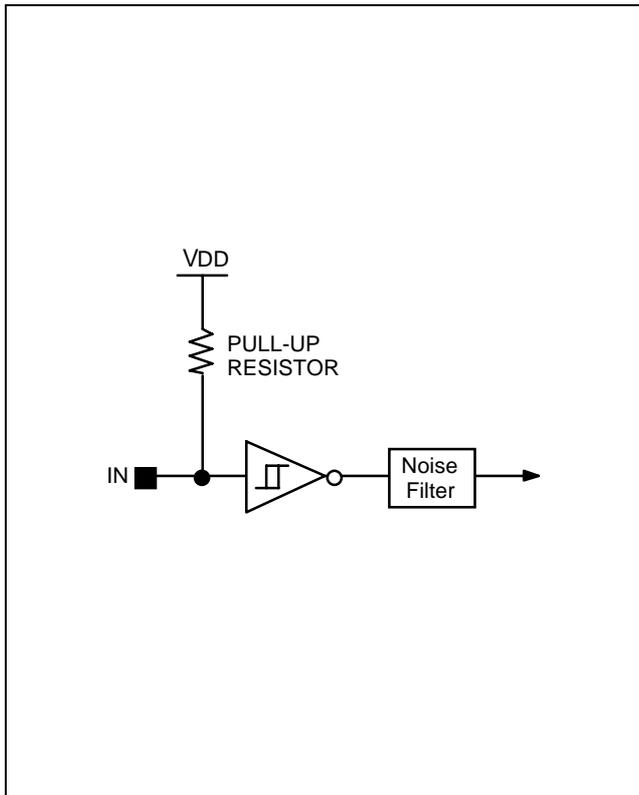
**Figure 1-4. Pin Circuit Type A (RESET)**
