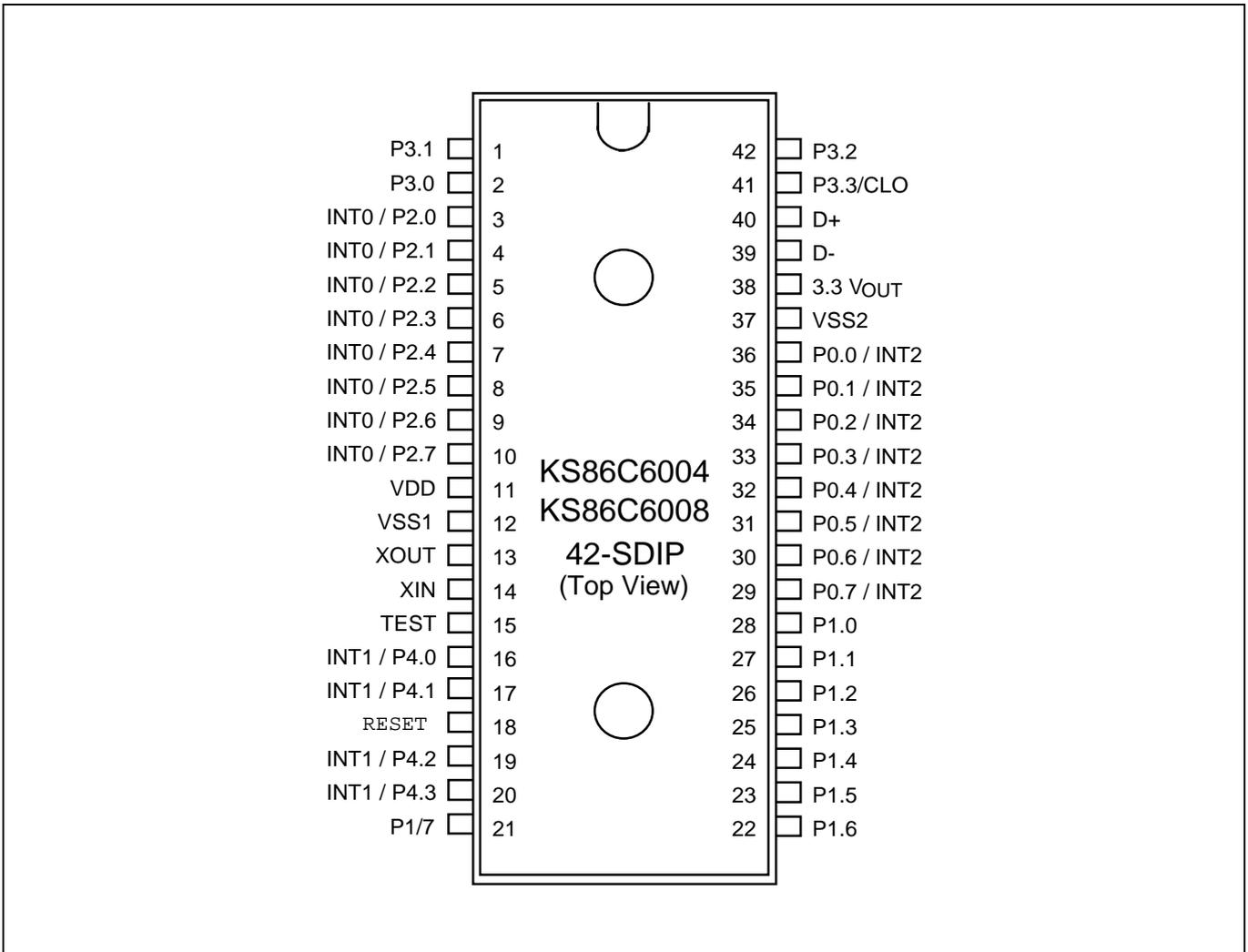
**Figure 1-2. Pin Assignment Diagram (42-Pin SDIP Package)**
