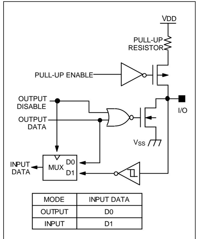
**Figure 1-5. Pin Circuit Type B (Ports 0, 1 and 2)**
