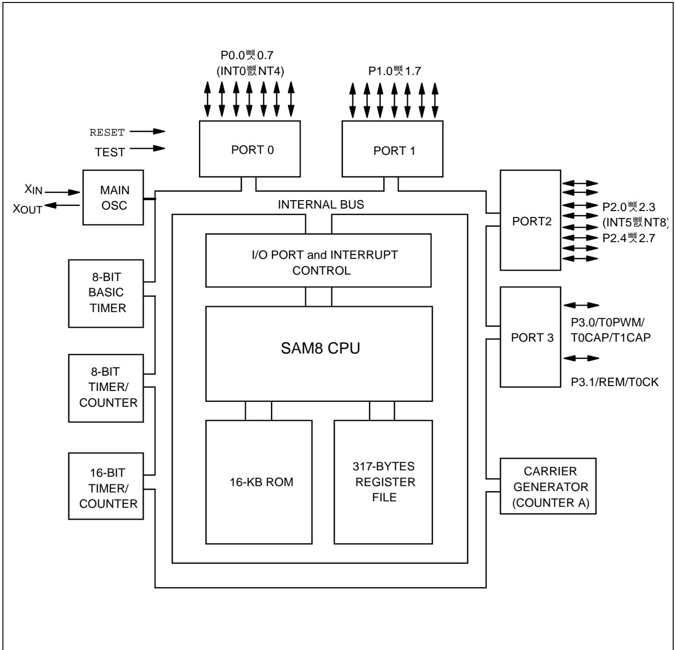
Figure 1-2. Block Diagram
