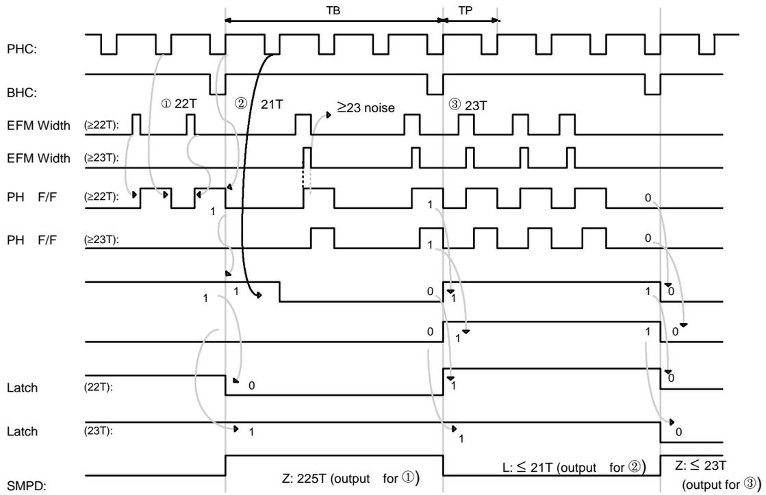
Fig. 18 The timing chart of SMSD output when gain is 'H'
