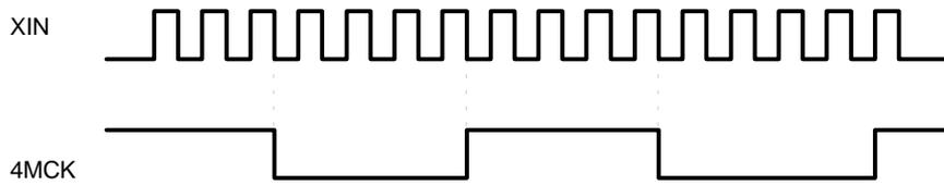
3) Using the X'tal osc of 8.4682 MHz, Timing Chart (Sel = 1)
