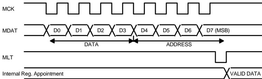
Fig. 3 **mCOM DATA INPUT TIMING CHART**
