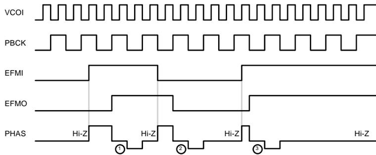
**Fig. 7 EFM Phase Detection Timing Chart**
