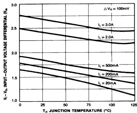
Figure 4. Dropout Voltage
