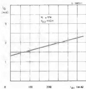
Fig. 7 - Quiescent current vs. input voltage
