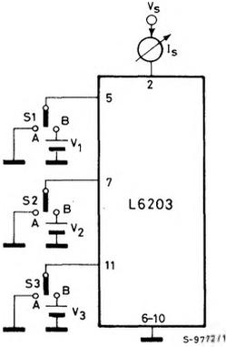
Fig. 11 - Leakage current
