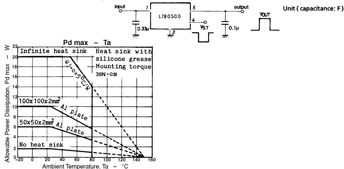
**Equivalent Circuit Block Diagram**
