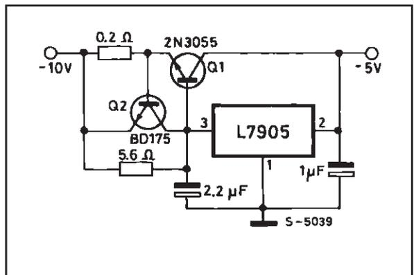
Figure 5 : Typical ECL System Power Supply (- 5.2V/4A).
