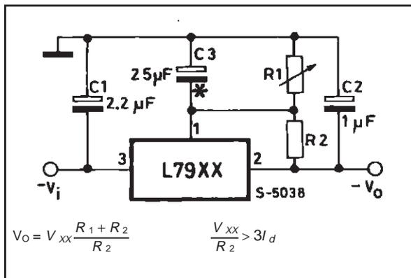
C3 Optional for improved transient response and ripple rejection.
