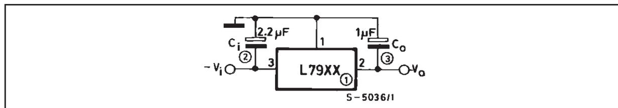
**ELECTRICAL CHARACTERISTICS FOR L7905A** (refer to the test circuits,  $T_j = 0$  to  $125$  °C,  $V_i = -10V$ ,  $I_o = 500$  mA,  $C_i = 2.2$   $\mu$ F,  $C_o = 1$   $\mu$ F unless otherwise specified)
