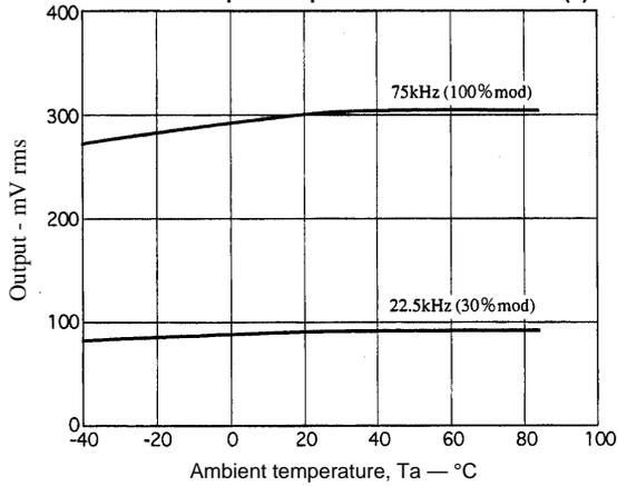
FM Antenna Input Temperature Characteristics (2)
