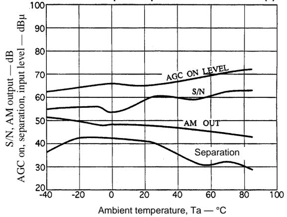
FM Antenna Input Temperature Characteristics (3)
