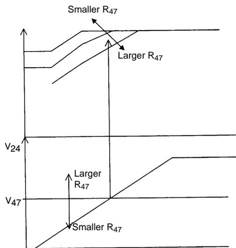
By comparing the pin 47 mute on adjustment voltage to the S-meter voltage (V<sub>24</sub>), the muting on point can be adjusted.
