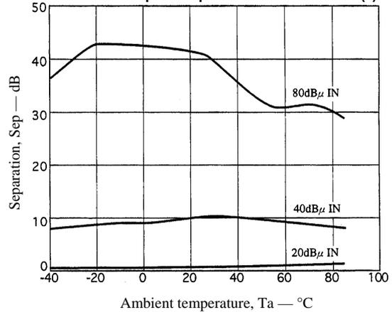
FM Antenna Input Temperature Characteristics (5)
