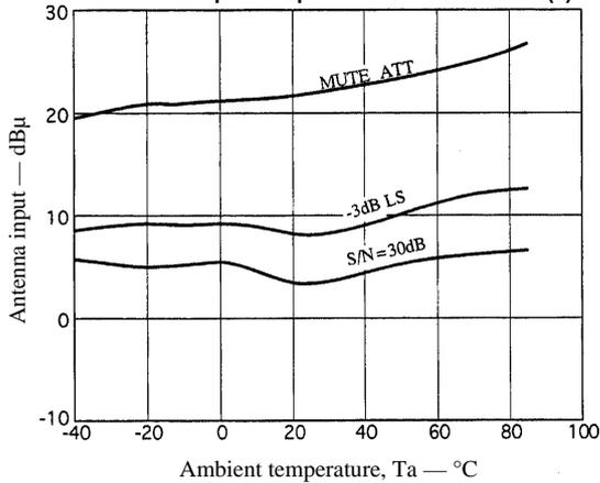
FM Antenna Input Temperature Characteristics (4)
