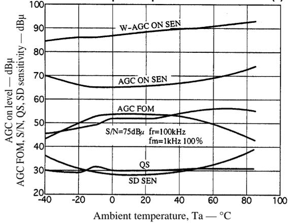
AM Antenna Input Temperature Characteristics (2)
