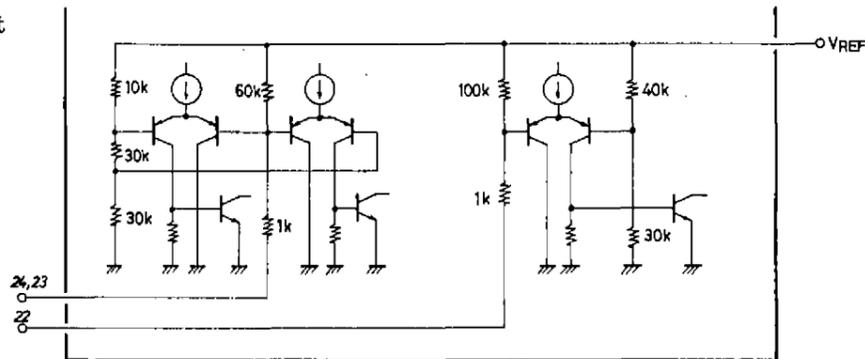
Input circuit of control pins (22, 23, 24) is shown above.
