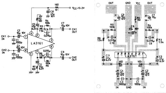
Unit (resistance: Ω, capacitance: F)
