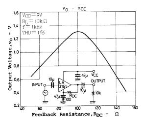
Unit (resistance: Ω, capacitance: F)
