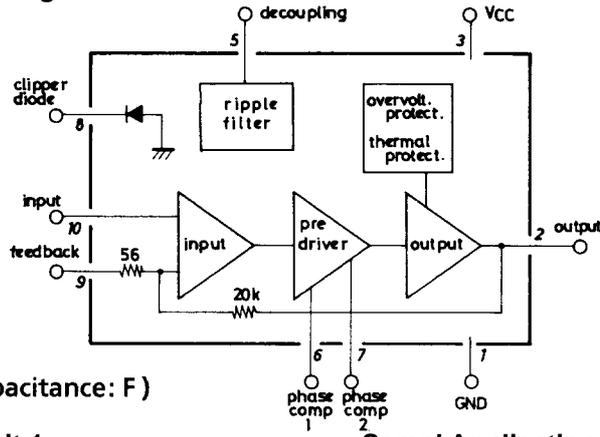
Unit (resistance:  $\Omega$ , capacitance: F)
