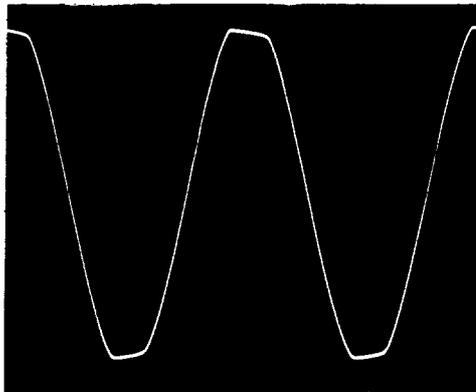
Pop noise waveform at the time of power switch OFF ( $V_{CC} = 16V$ ,  $R_L = 8\Omega$ , quiescent)
