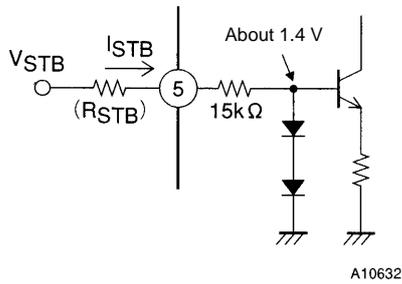
Pin 5 in this IC is the standby pin, and applying a voltage of 2.0 V or higher will activate this function. The pin 5 influx current for an applied voltage of 5 V will be about 240  $\mu$ A.
