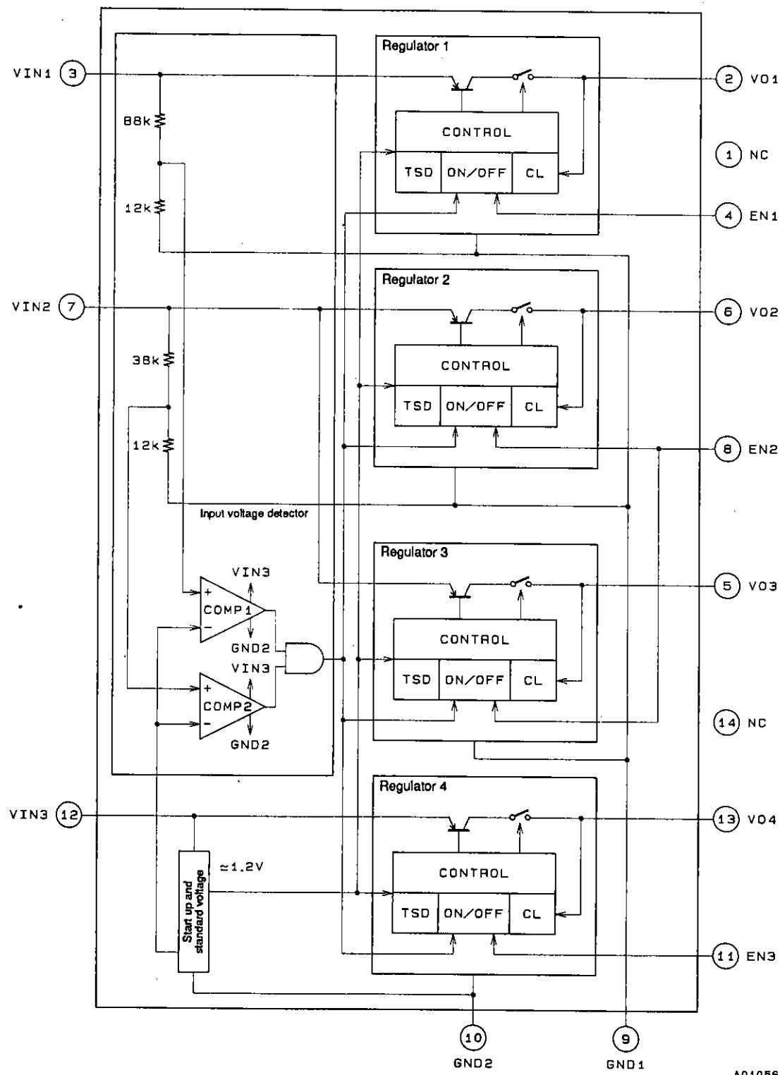
TSD: Thermal Shutdown Circuit
