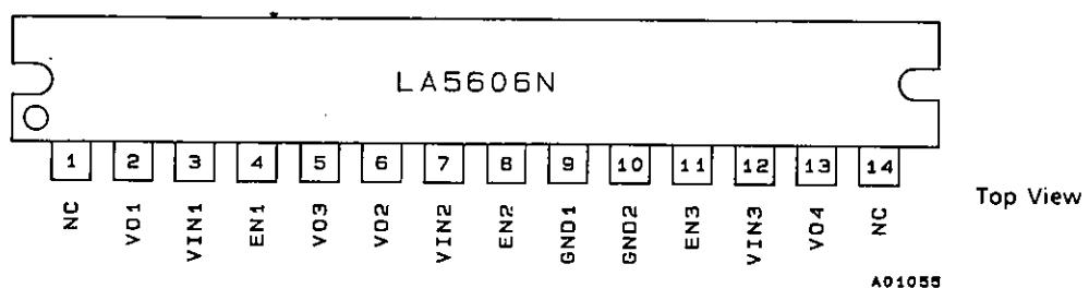
Note: The NC pins should not be used (No. 1 and No. 14 in the pin layout).
