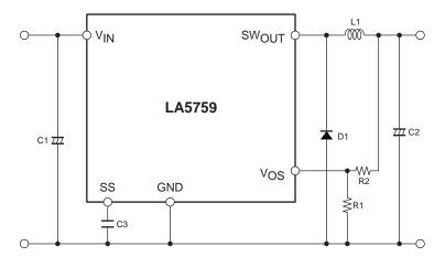
Notes: C3 is for the soft start function. Delete C3 and keep the SS pin open when the soft function is not necessary.
