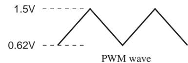
$$PWMduty = \frac{V_{OUT}}{V_{IN} - V_{sat} + VF} = 23 \%$$
