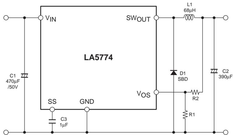
Notes: C3 is for the soft start function. Delete C3 and keep the SS pin open when the soft start function is not necessary.
