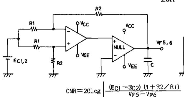
$$\text{CMR} = 20 \log \left| \frac{(E_{K1} - E_{K2})(1 + R_2/R_1)}{V_{F5.6} - V_{F6}} \right|$$
