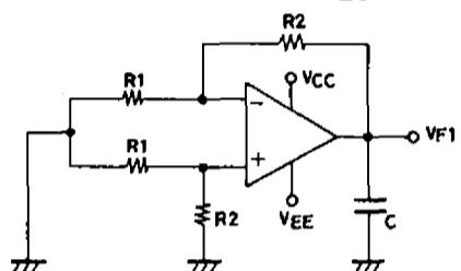
$$V_{IO} = \frac{V_{F1}}{1 + R_2/R_1}$$
