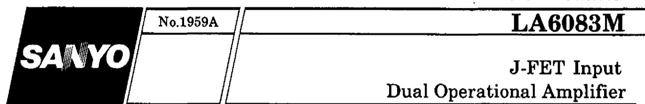
The LA6083M is a J-FET input dual operational amplifier. Application areas include general-purpose control equipment, measuring equipment (very low current measurement, long-integrating circuit, sample & hold circuit, impedance converter, etc.).
