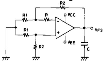
$$I_B = \frac{V_{F4} - V_{F3}}{2R(1 + R_2/R_1)}$$
