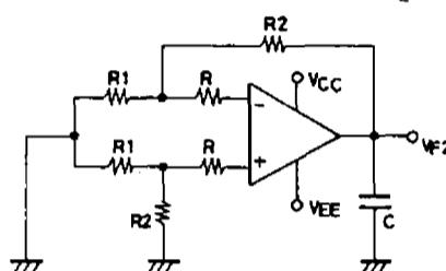
$$I_{IO} = \frac{V_{F2} - V_{F1}}{R(1 + R_2/R_1)}$$
