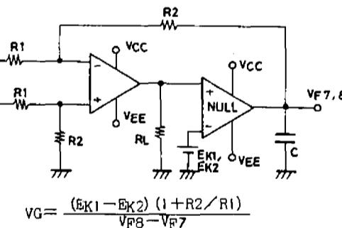
$$VG = \frac{(E_{K1} - E_{K2})(1 + R_2/R_1)}{V_{F8} - V_{F7}}$$
