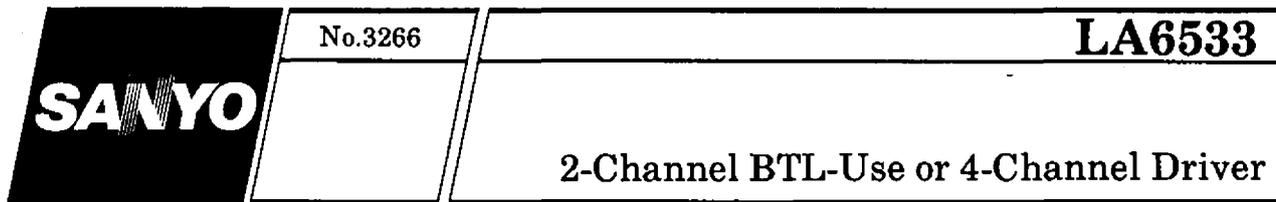
The LA6533 is a 2-channel BTL-use driver designed for compact disc pickup actuation or a 4-channel driver for general-purpose applications.
