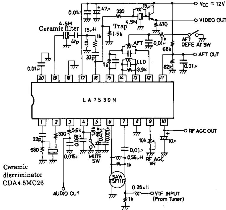
Unit (resistance:Ω, capacitance:F)
