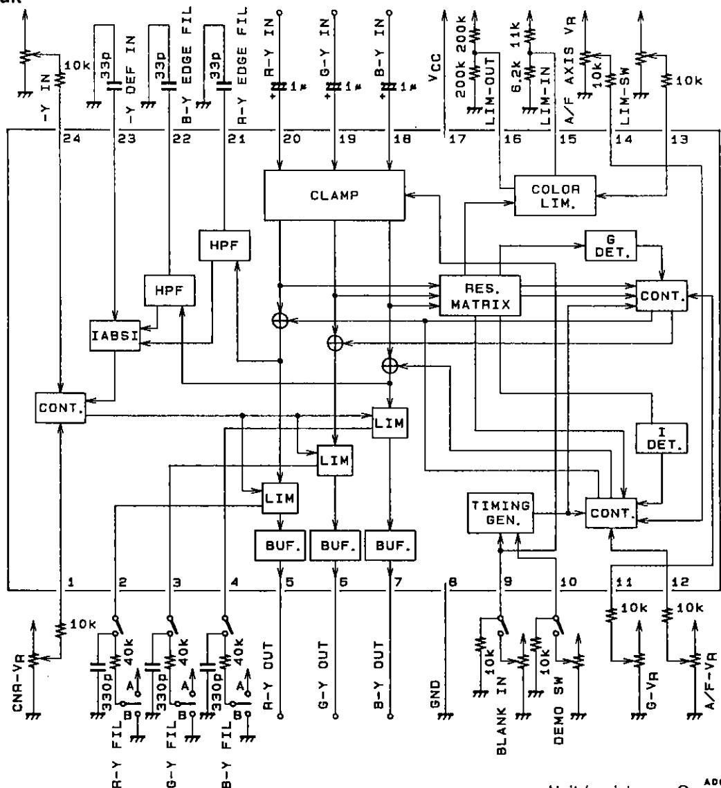
Note: All  $V_R$ s are 10 k $\Omega$  variable resistors
