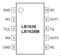
Note: both ground pins must be grounded.
