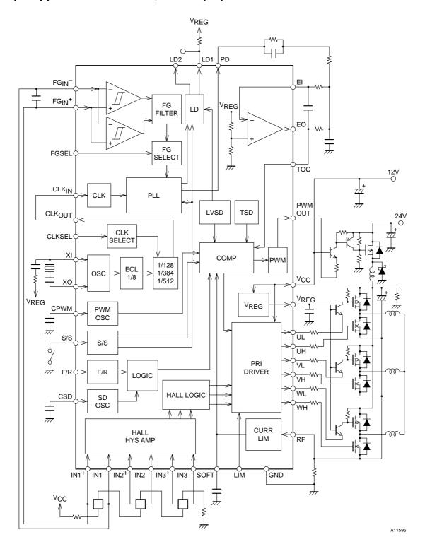
Note: For applications where the motor has variable speed and control at low motor voltages is required, the base voltage of the output interface transistor must be made low. In this case, a P-channel FET which can be used at low gate voltages must be selected.
