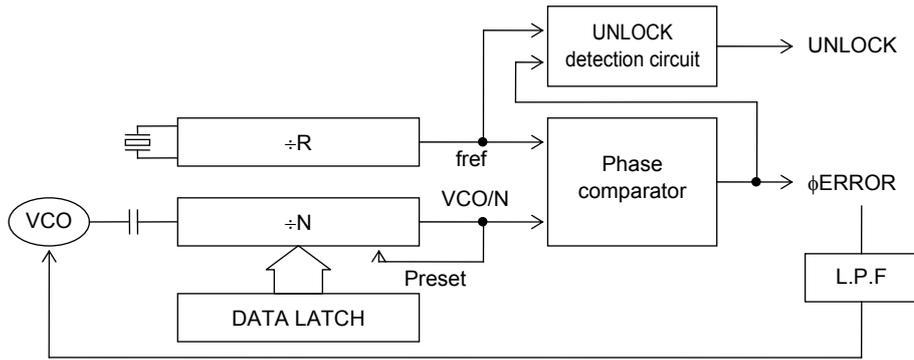
Figure 2 Circuit Structure
